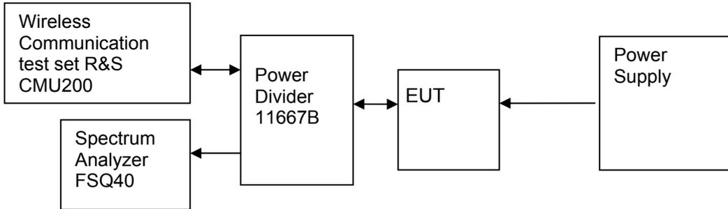
Figure 6. Test Set-up
