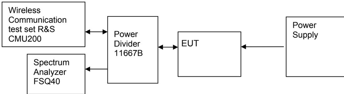
Figure 1. Test Set-up
