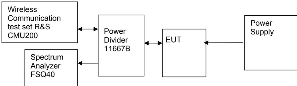
Figure 2. Test Set-up
