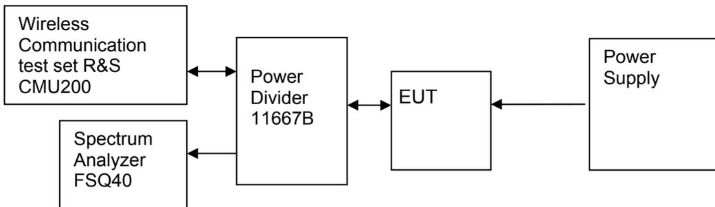
Figure 7. Test Set-up
