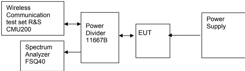
Figure 5. Test Set-up
