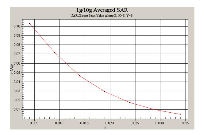
Figure 31 Z-Scan at power reference point (Right Hand Tilt 15° Open GSM 1900 Channel 512)
