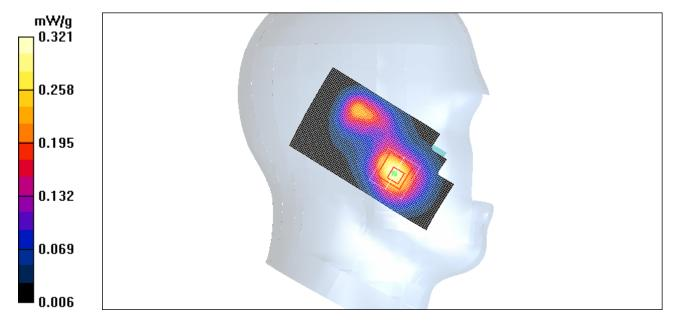
Figure 64 Left Hand Touch Cheek Close GSM 1900 Channel 512
