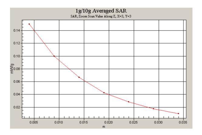
Figure 59 Z-Scan at power reference point (Body, Towards Phantom, Open GSM 1900 GPRS Channel 512)
