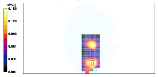
Figure 58 Body, Towards Phantom, Open GSM 1900 GPRS Channel 512
