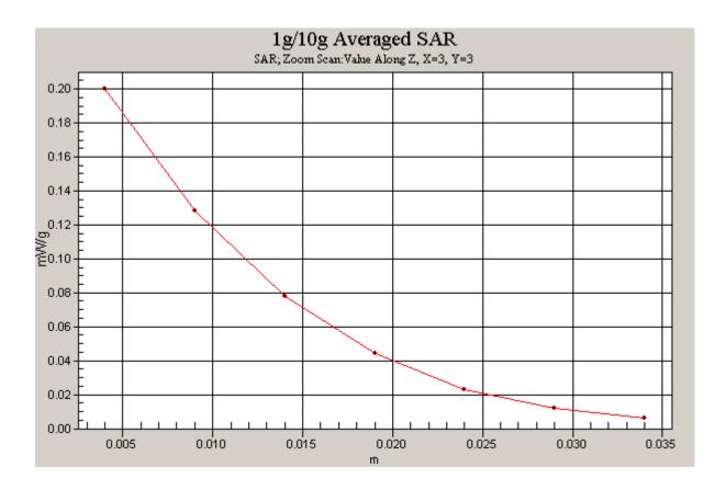
Figure 35 Z-Scan at power reference point (Body, Towards Ground, Open GSM 1900 Channel 661)
