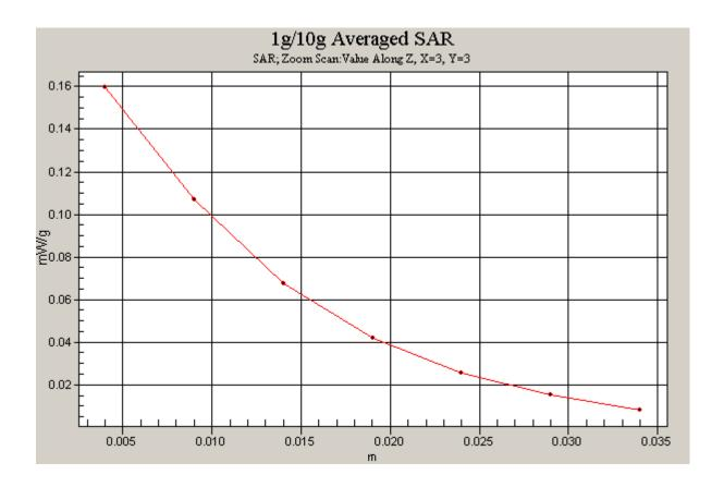
Figure 21 Z-Scan at power reference point (Right Hand Touch Cheek Open GSM 1900 Channel 810)
