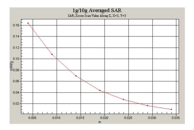
Figure 55 Z-Scan at power reference point (Body, Towards Phantom, Open GSM 1900 GPRS, Channel 810)
