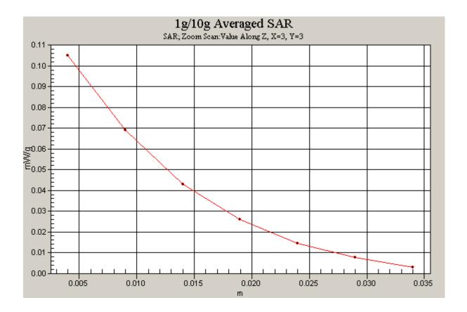
Figure 27 Z-Scan at power reference point (Right Hand Tilt 15° Open GSM 1900 Channel 810)
