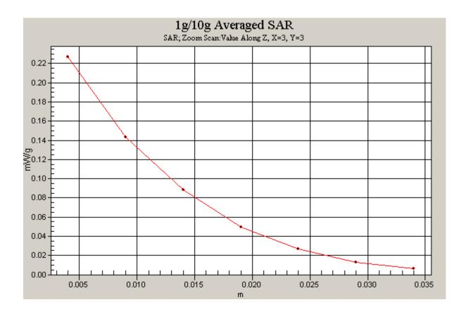
Figure 45 Z-Scan at power reference point (Body with Earphone, Towards Ground, Open GSM 1900, Channel 810)
