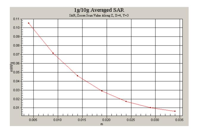
Figure 19 Z-Scan at power reference point (Left Hand Tilt 15° Open GSM 1900 Channel 512)
