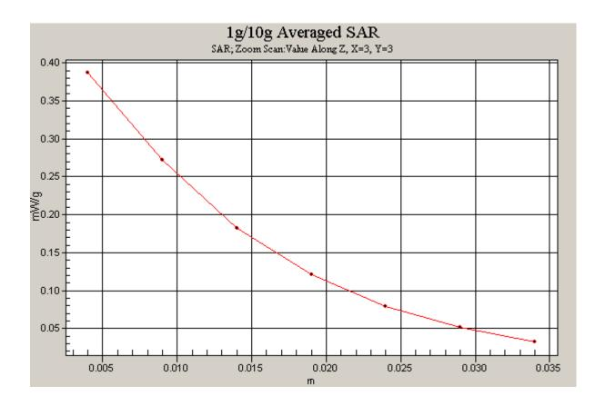
Figure 61 Z-Scan at power reference point (Left Hand Touch Cheek Close GSM 1900 Channel 810)
