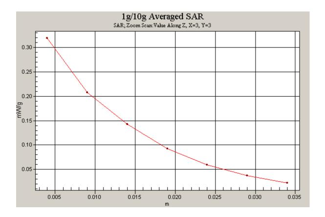
Figure 51 Z-Scan at power reference point (Body, Towards Ground, Open GSM 1900 GPRS Channel 661)
