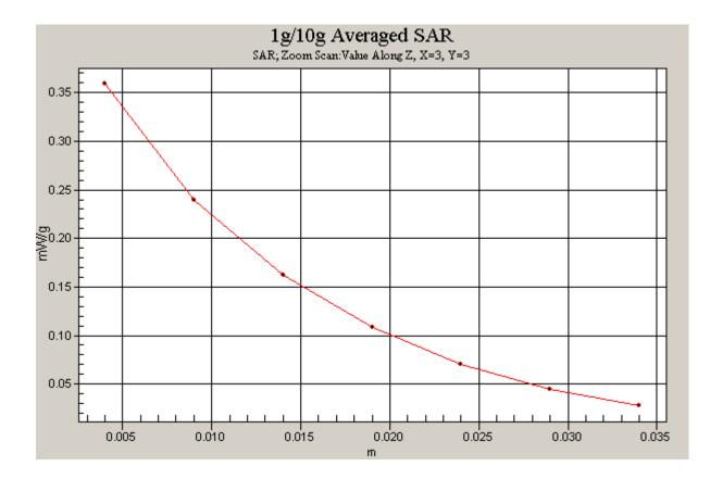
Figure 53 Z-Scan at power reference point (Body, Towards Ground, Open GSM 1900 GPRS Channel 512)
