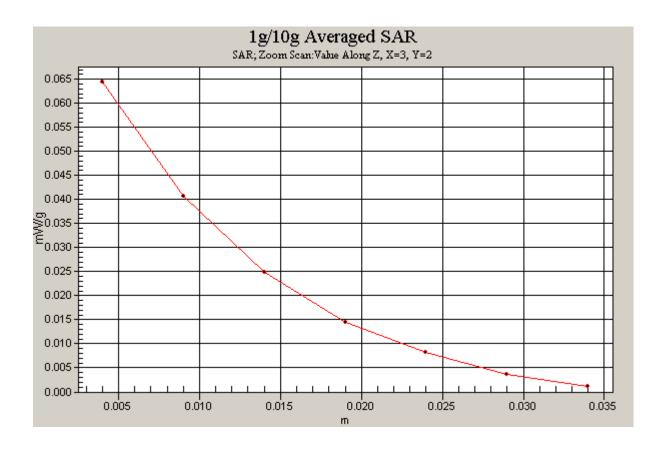
Figure 39 Z-Scan at power reference point (Body, Towards Phantom, Open GSM 1900 Channel 810)
