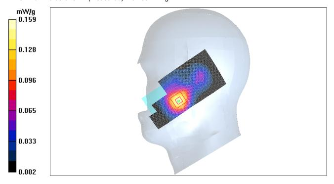
Figure 24 Right Hand Touch Cheek Open GSM 1900 Channel 512
