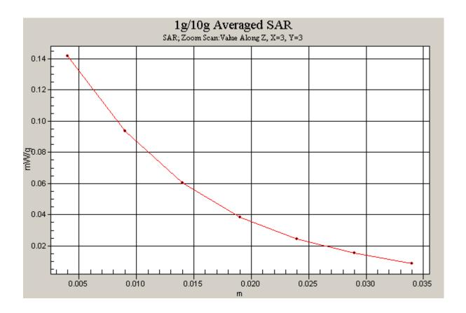
Figure 57 Z-Scan at power reference point (Body, Towards Phantom, Open GSM 1900 GPRS Channel 661)
