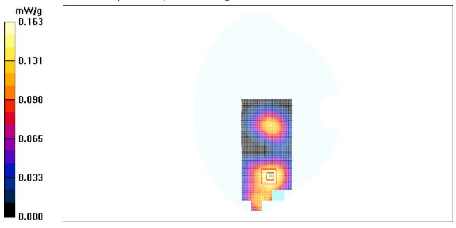
Figure 54 Body, Towards Phantom, Open GSM 1900 GPRS, Channel 810
