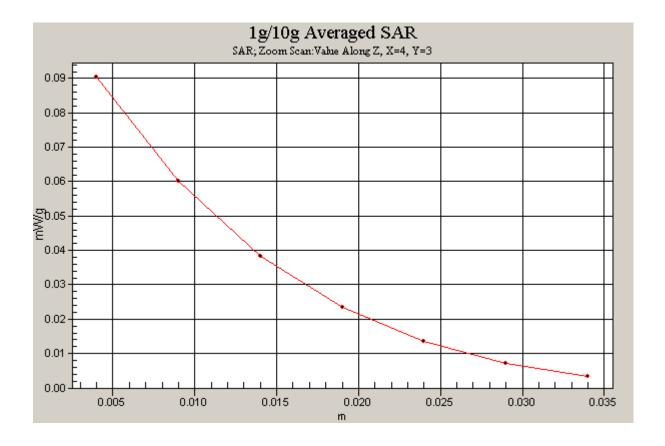
Figure 29 Z-Scan at power reference point (Right Hand Tilt 15° Open GSM 1900 Channel 661)
