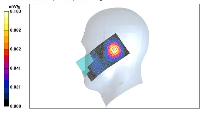
Figure 30 Right Hand Tilt 15° Open GSM 1900 Channel 512
