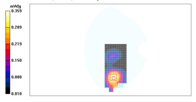
Figure 52 Body, Towards Ground, Open GSM 1900 GPRS Channel 512
