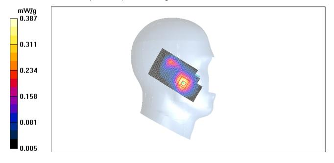
Figure 60 Left Hand Touch Cheek Close GSM 1900 Channel 810
