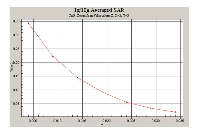
Figure 49 Z-Scan at power reference point (Body, Towards Ground, Open GSM 1900 GPRS, Channel 810)
