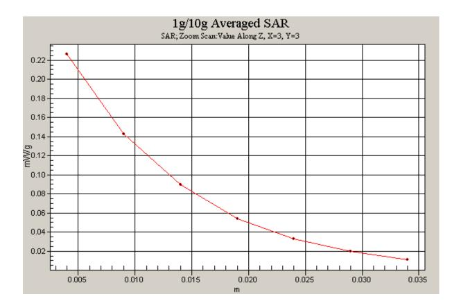
Figure 47 Z-Scan at power reference point (Body with Bluetooth earphone, Towards Ground, Open GSM 1900, Channel 810
