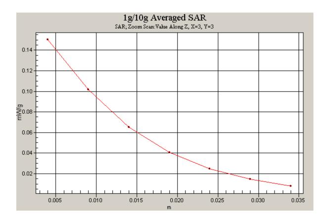
Figure 23 Z-Scan at power reference point (Right Hand Touch Cheek Open GSM 1900 Channel 661)
