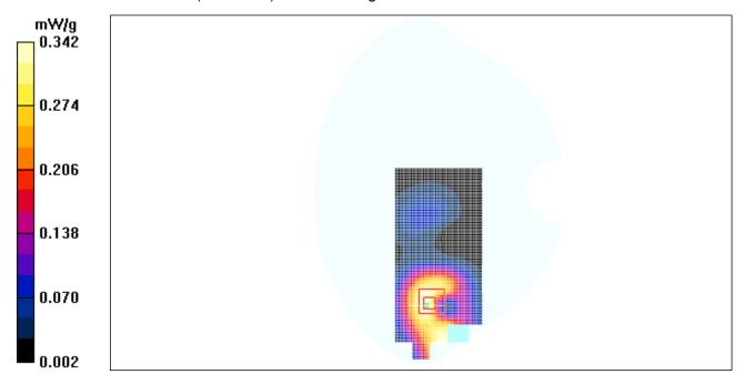
Figure 48 Body, Towards Ground, Open GSM 1900 GPRS, Channel 810
