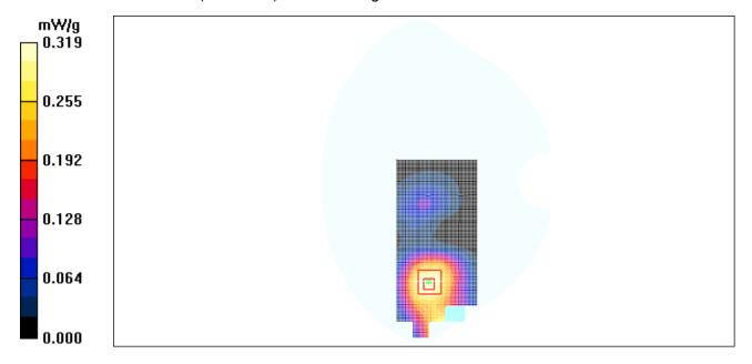
Figure 50 Body, Towards Ground, Open GSM 1900 GPRS Channel 661
