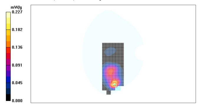
Figure 44 Body with Earphone, Towards Ground, Open GSM 1900, Channel 810
