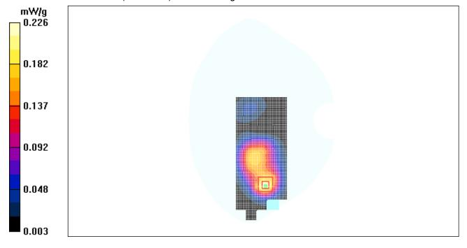
Figure 46 Body with Bluetooth earphone, Towards Ground, Open GSM 1900, Channel 810
