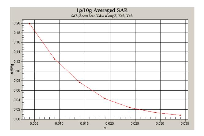
Figure 37 Z-Scan at power reference point (Body, Towards Ground, Open GSM 1900 Channel 512)
