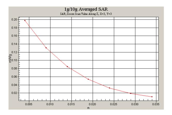
Figure 67 Z-Scan at power reference point (Left Hand Tilt 15°Close GSM 1900 Channel 810)
