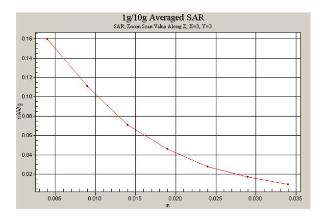
Figure 25 Z-Scan at power reference point (Right Hand Touch Cheek Open GSM 1900 Channel 512)
