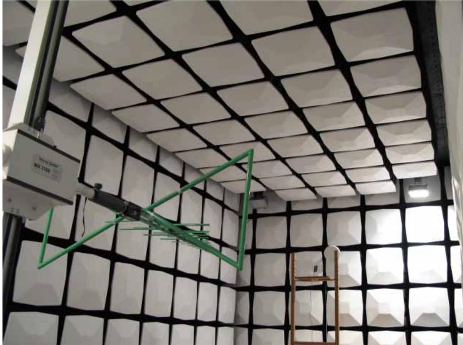
Radiated Spurious Emission(30MHz~2000MHz)
