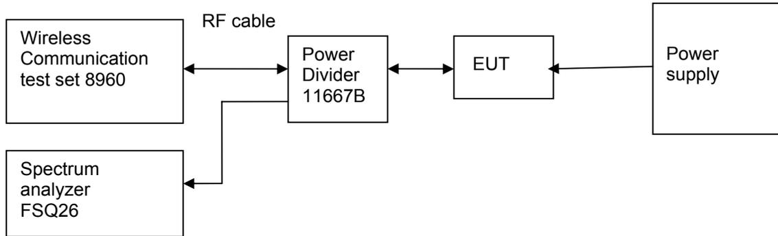
Figure 6. Test Set-up
