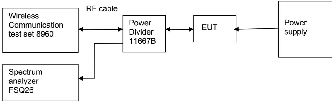
Figure 5. Test Set-up
