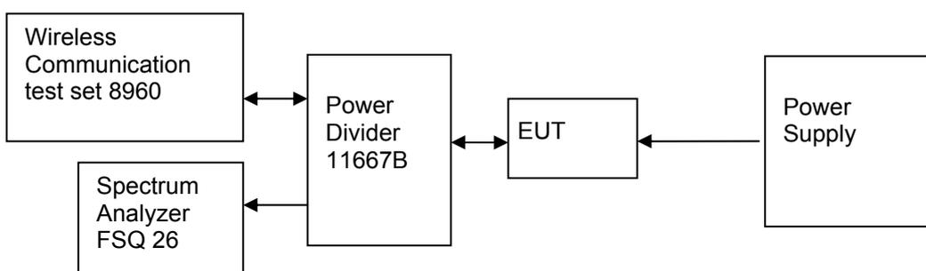
Figure 4. Test Set-up
