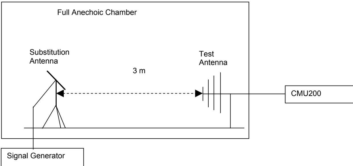
Figure 1. Test Set-up
