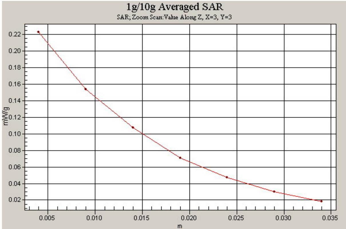
Fig. 86 Z-Scan at power reference point (Body, Towards the ground, PCS 1900MHz+EGPRS, CH512)
