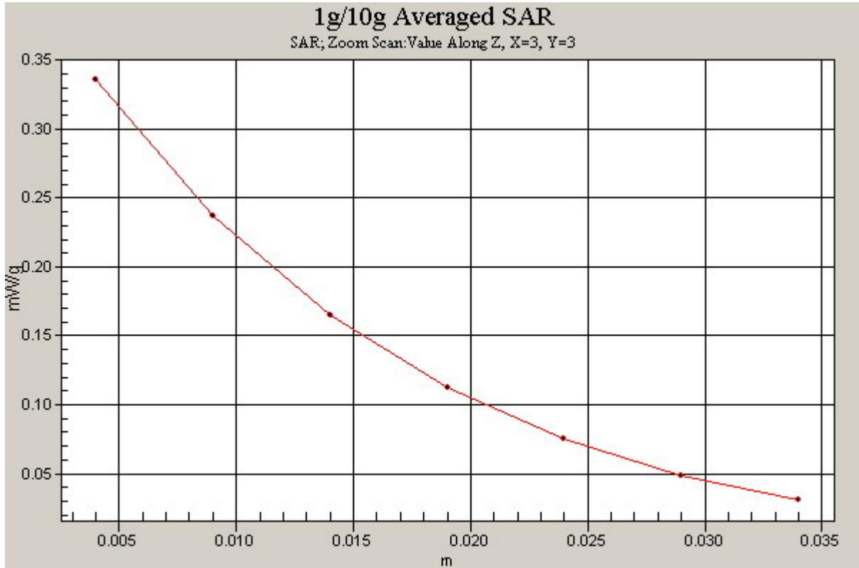
**Fig. 78 Z-Scan at power reference point
