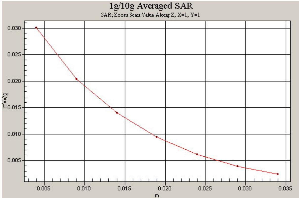
Fig. 68 Z-Scan at power reference point (PCS 1900MHz CH661)
