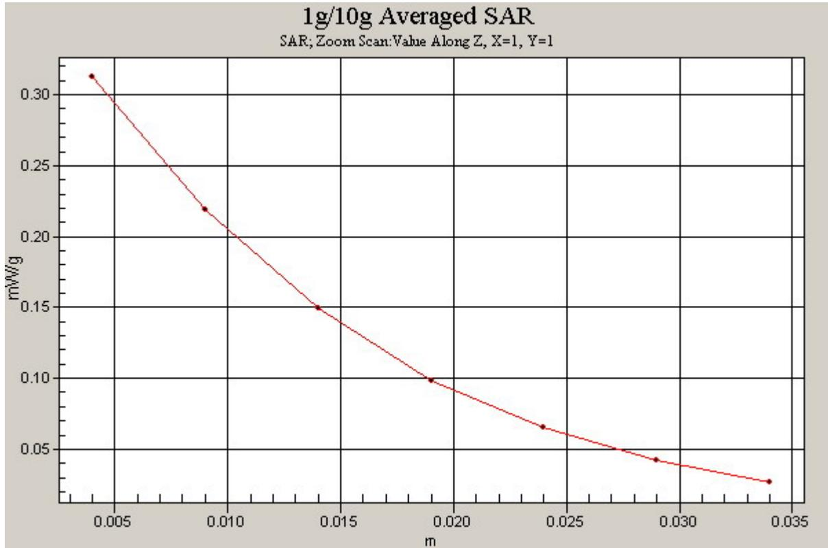
Fig. 74 Z-Scan at power reference point (Body, Towards the ground, PCS 1900MHz, CH661)
