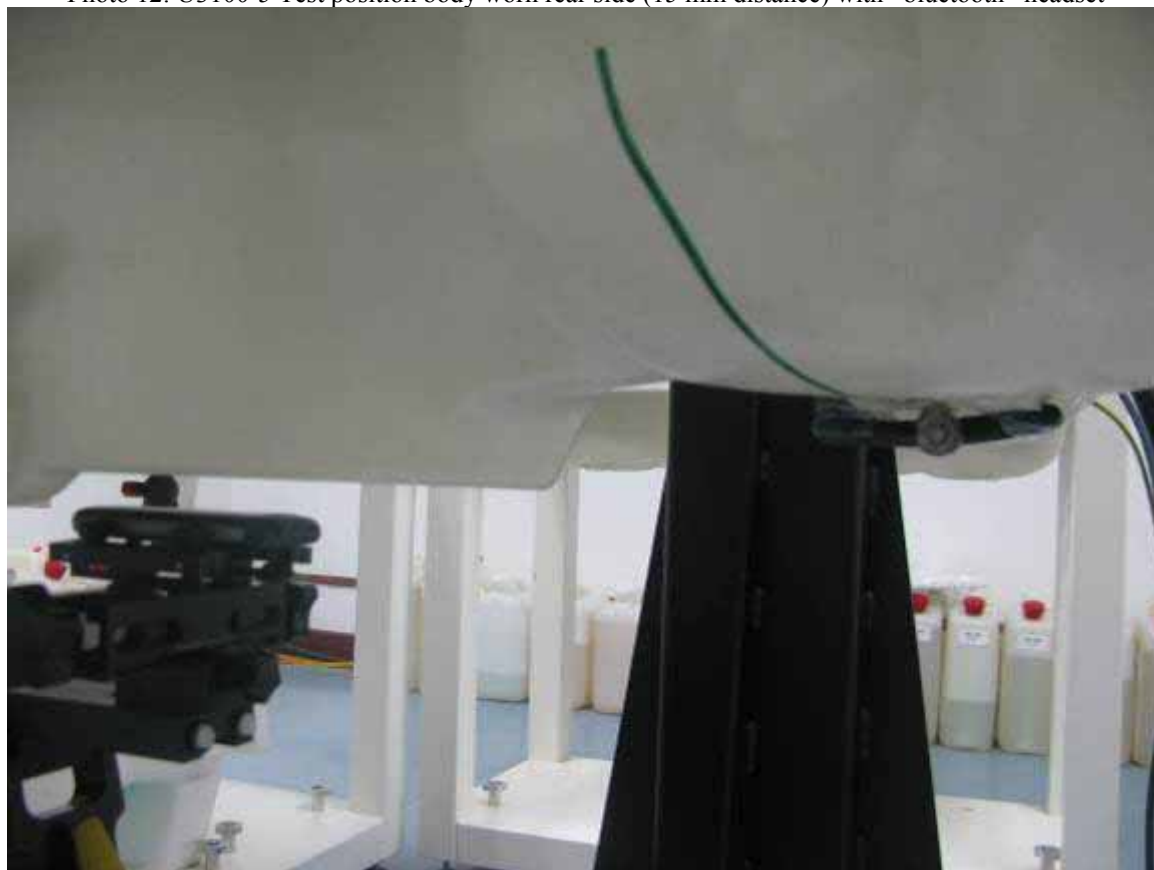
Photo 12: U3100-5 Test position body worn rear side (15 mm distance) with bluetooth headset
