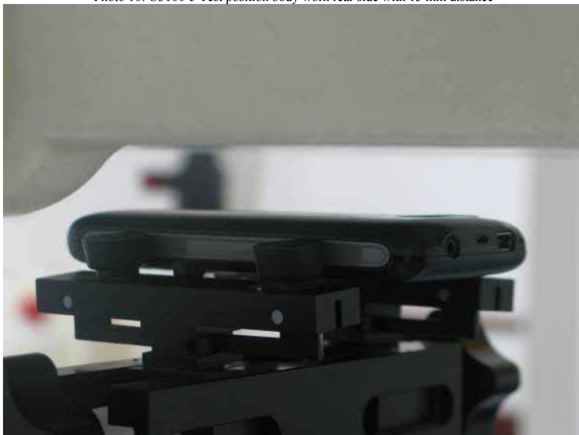
Photo 10: U3100-5 Test position body worn rear side with 15 mm distance
