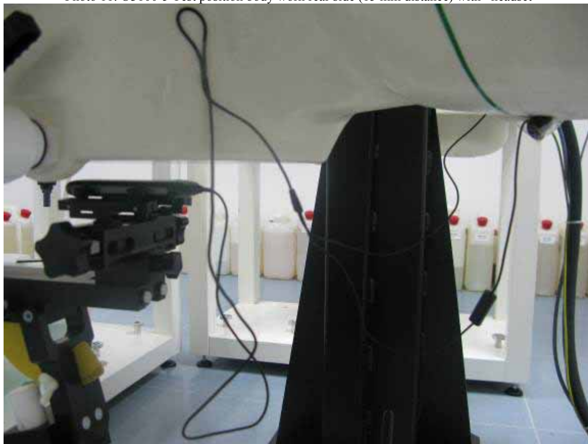
Photo 12: U3100-5 Test position body worn rear side (15 mm distance) with bluetooth headset
