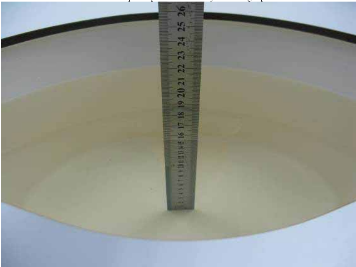
Photo 14: Liquid depth 900 MHz body simulating liquid
