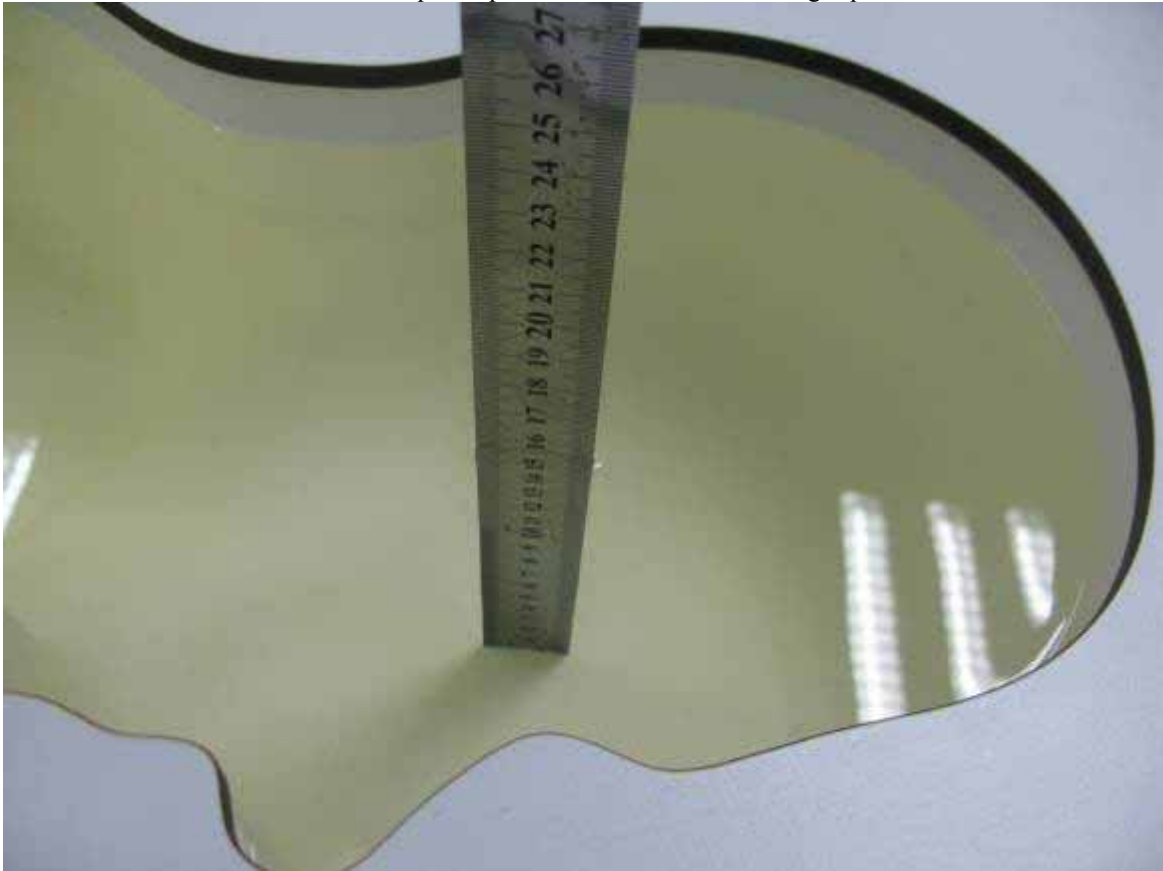
Photo 15: Liquid depth 1950 MHz head simulating liquid
