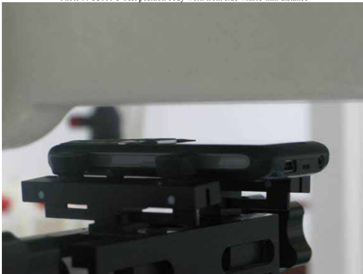
Photo 10: U3100-5 Test position body worn rear side with 15 mm distance
