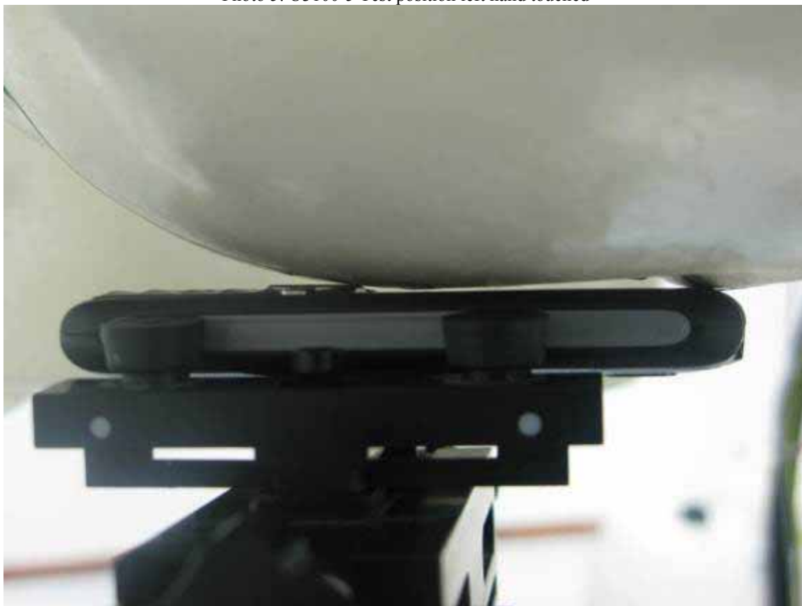
Photo 6: U3100-5 Test position left hand tilted 15°
