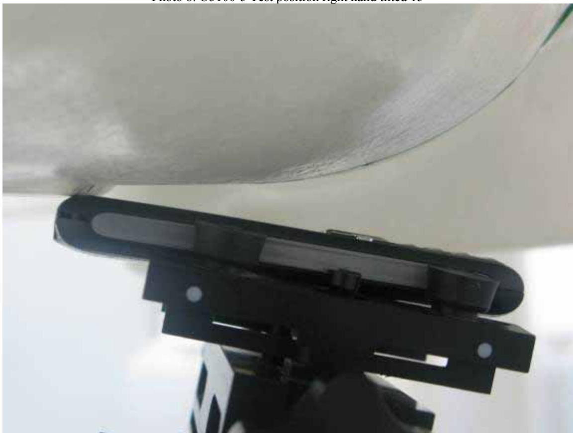
Photo 8: U3100-5 Test position right hand tilted 15°
