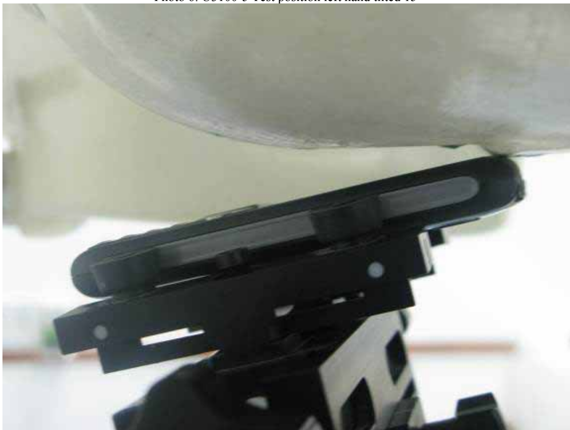
Photo 6: U3100-5 Test position left hand tilted 15°
