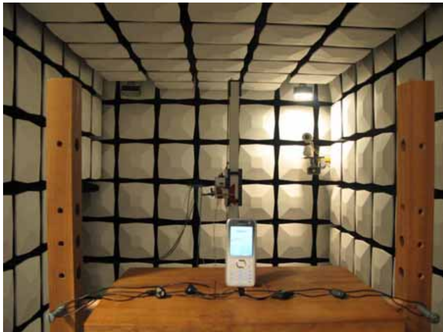
Radiated Spurious Emission (2GHz to18GHz)
