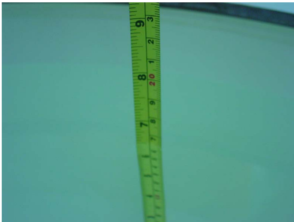
Picture B3 Liquid depth in the Flat Phantom (PCS 1900MHz)
