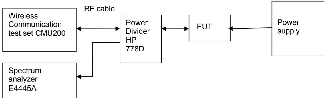
Figure 6. Test Set-up
