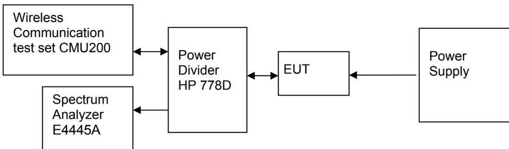
Figure 4. Test Set-up
