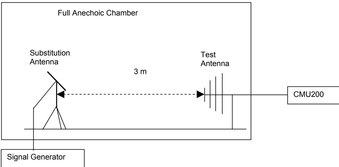
Figure 1. Test Set-up
