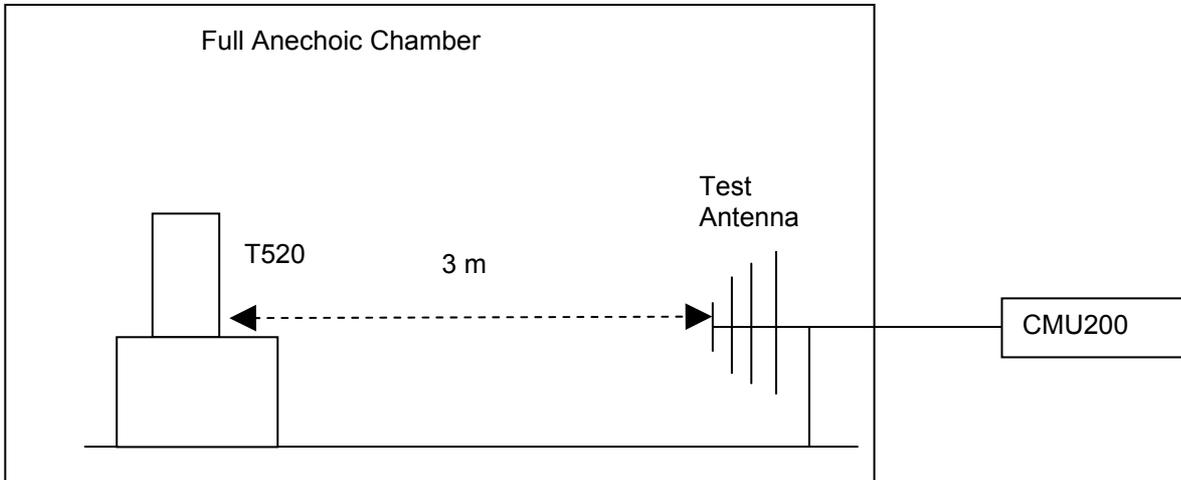
**Step 2: Substitution method to verify the maximum ERP**
