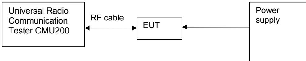
Figure 2. Test Set-up
