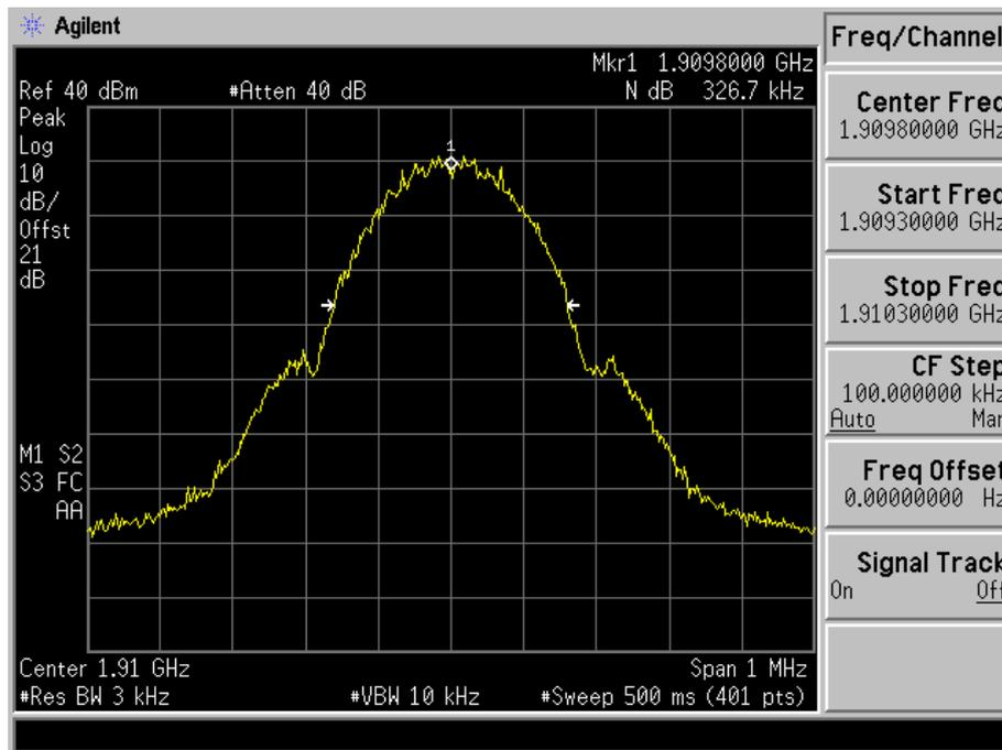
**5. Spurious Emission At Antenna Terminals (+/-1MHz)**
