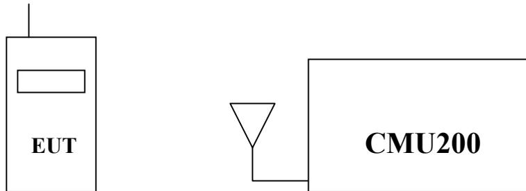
(b) Configuration of Conducted measurement
