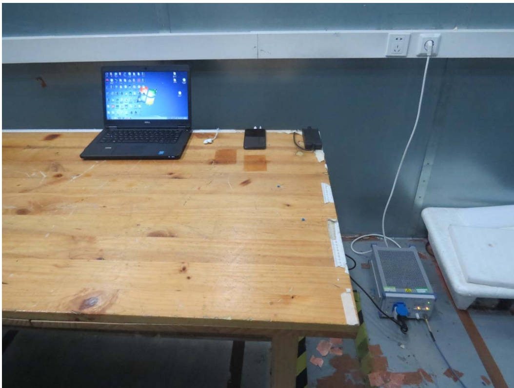
Picture 2 Conducted Emission Test Setup
