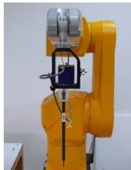
Figure 3. EX3DV4 E-field probe
