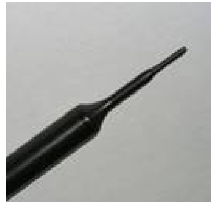
Figure 2. EX3DV4 E-field Probe
