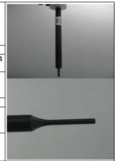
Isotropic E-Field Probe EX3DV4 for Dosimetric Measurements
