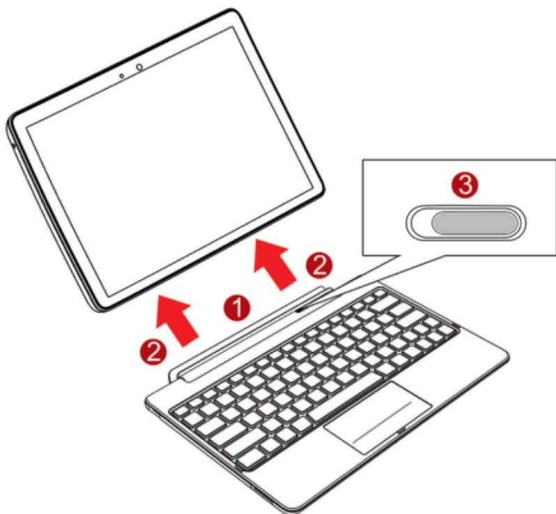
1. Rotate the hinge by 60 to 120 degrees to make the dock's opening face upward.
