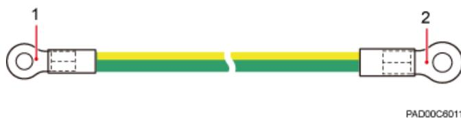
(1) OT terminal (M6, 16 mm<sup>2</sup> or 0.025 in.<sup>2</sup>)    (2) OT terminal (M8, 16 mm<sup>2</sup> or 0.025 in.<sup>2</sup>)
