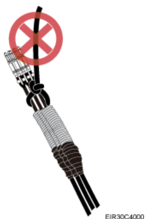
Figure 7-8 Incorrect binding method
