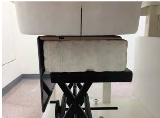
Fig.3 EUT Bottom side to flat phantom
