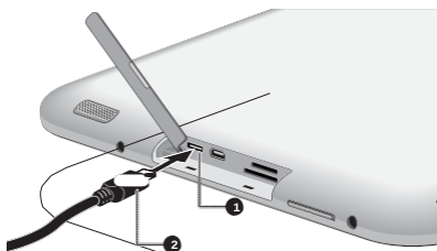
Figure 4-4 Connecting an USB cable
