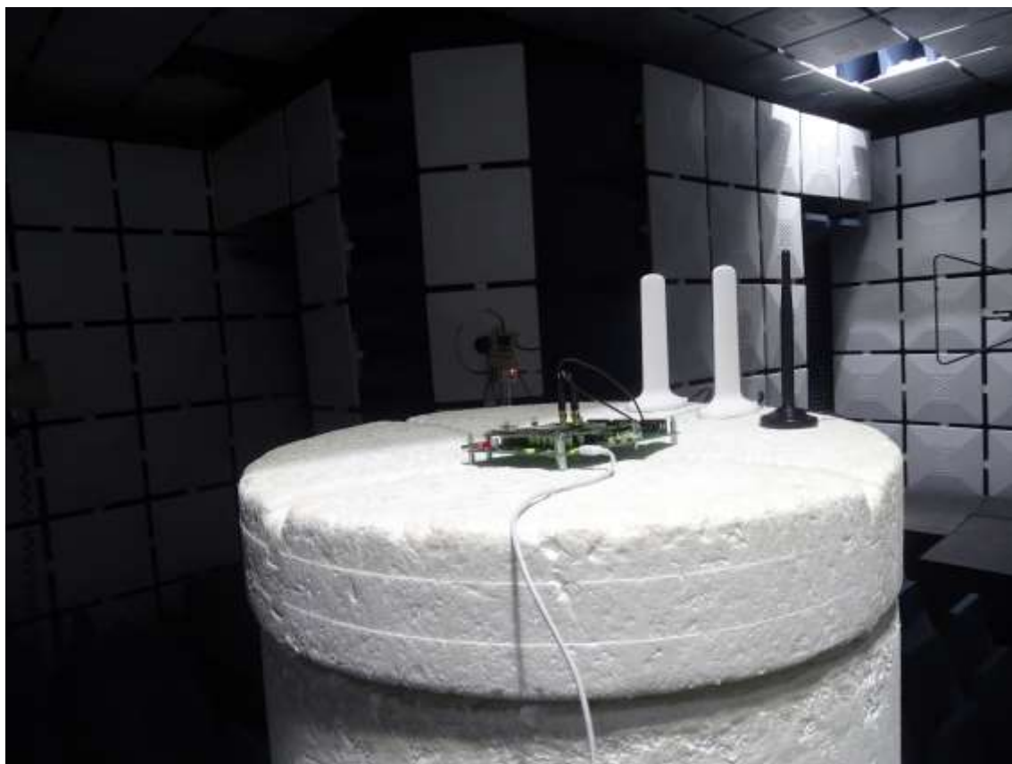
Radiated Spurious Emission (18GHz to26.5GHz)
