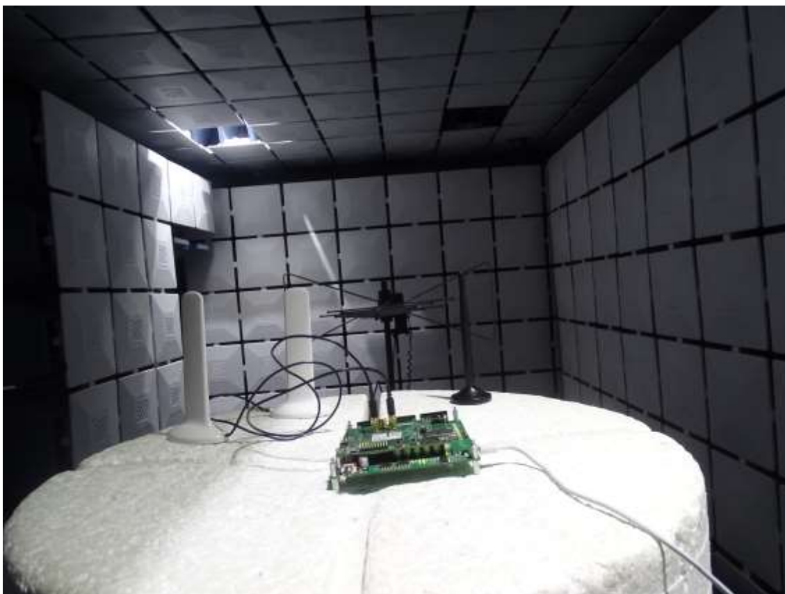
Radiated Spurious Emission (30MHz to 3GHz)
