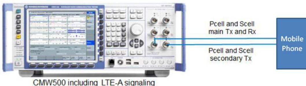
Table 44: Conducted power measurement setup of LTE CA per 3GPP TS 36.521-1 V10.5.0
