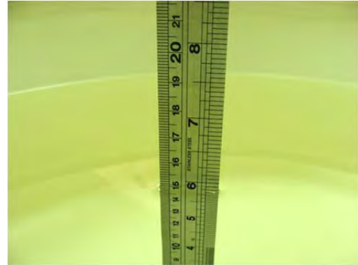
Fig 6.2 Photo of Liquid Height for Body SAR
