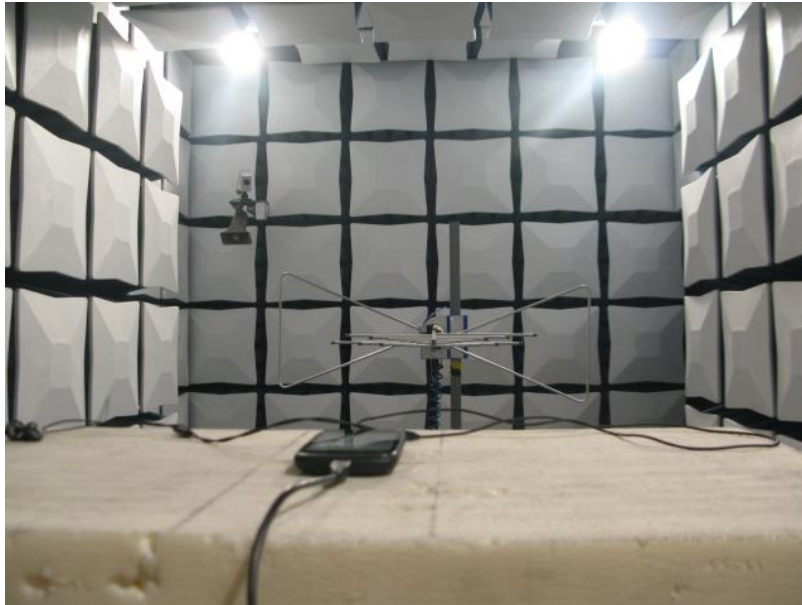
Radiated Spurious Emission (below 3GHz)
