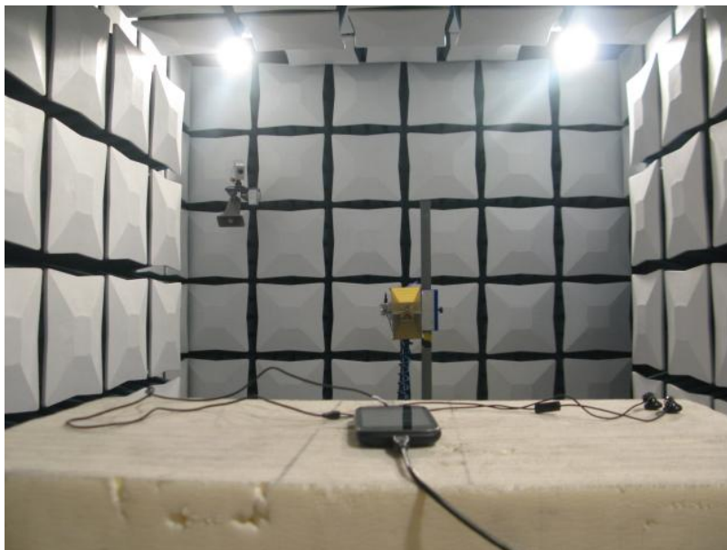
Radiated Spurious Emission (3GHz to18GHz)
