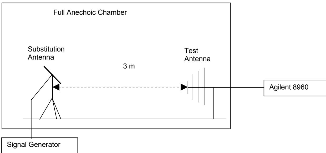
Figure 1. Test Set-up
