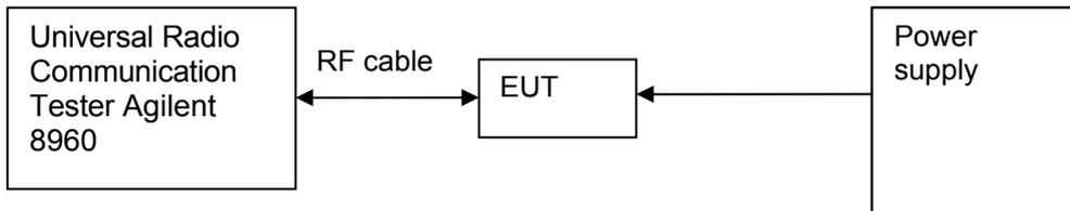
Figure 2. Test Set-up
