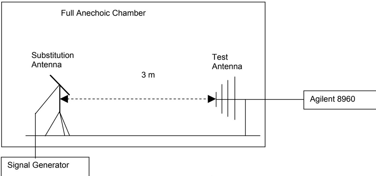
**Figure 1. Test Set-up**
