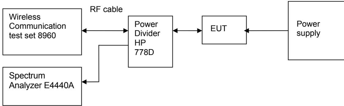
Figure 5. Test Set-up
