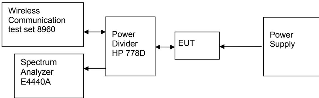
Figure 4. Test Set-up
