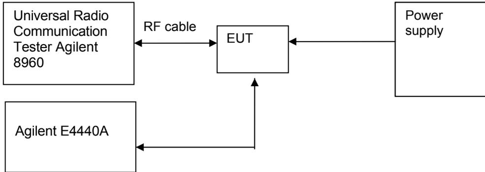
Figure 2. Test Set-up
