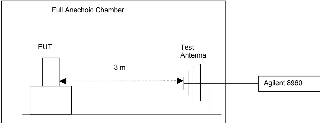
**Step 2: Substitution method to verify the maximum EIRP**
