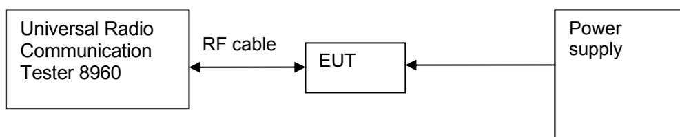
Figure 3. Test Set-up
