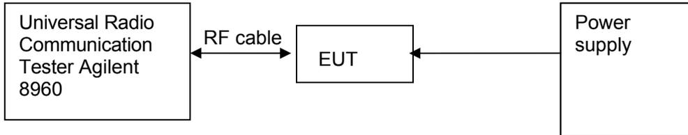
Figure 2. Test Set-up
