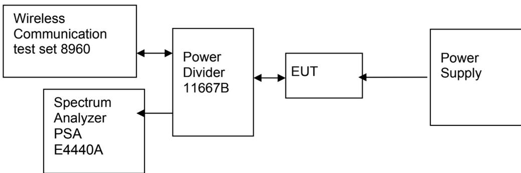
Figure 4. Test Set-up
