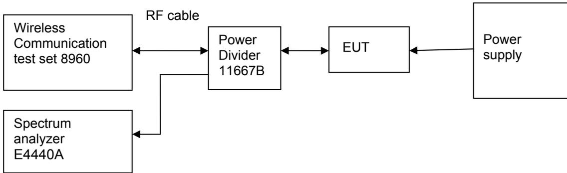
Figure 5. Test Set-up
