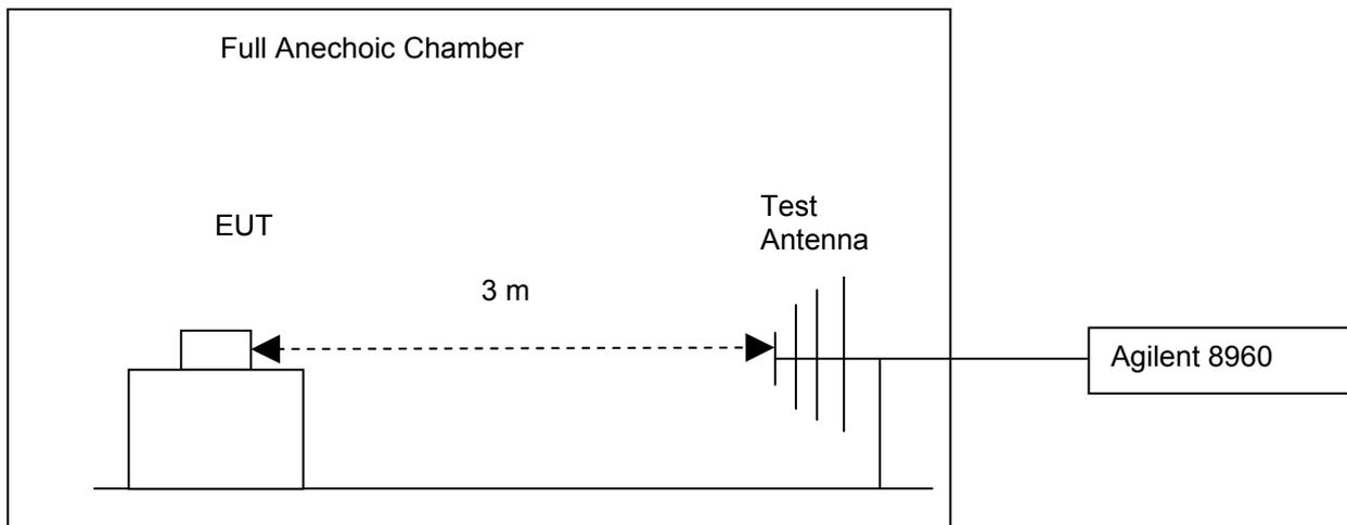
**Step 2: Substitution method to verify the maximum ERP**
