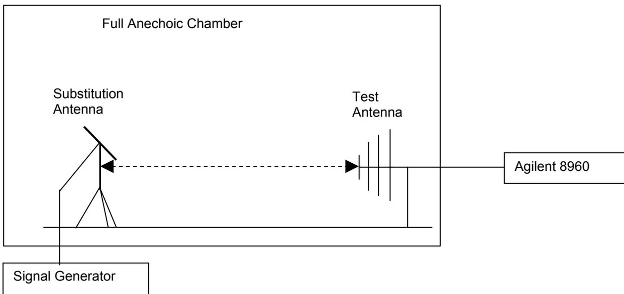
Figure 1. Test Set-up
