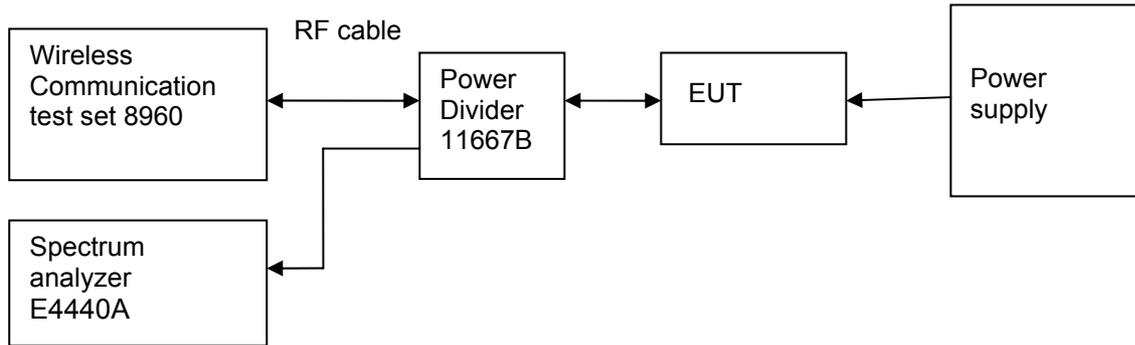
Figure 6. Test Set-up
