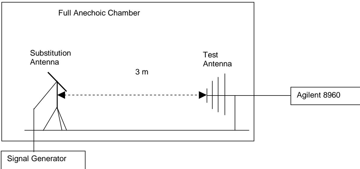
Figure 1. Test Set-up
