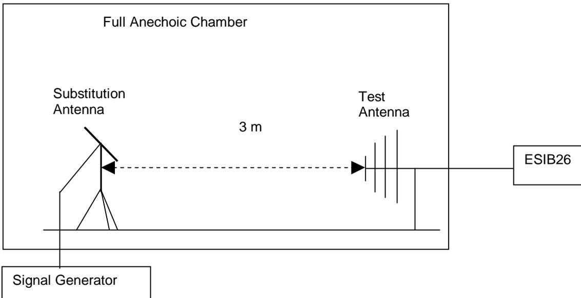
Figure 7. Test Set-up
