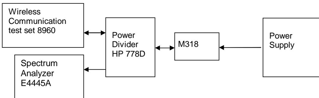
Figure 4. Test Set-up
