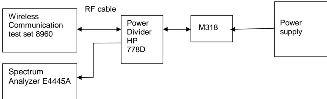
Figure 6. Test Set-up
