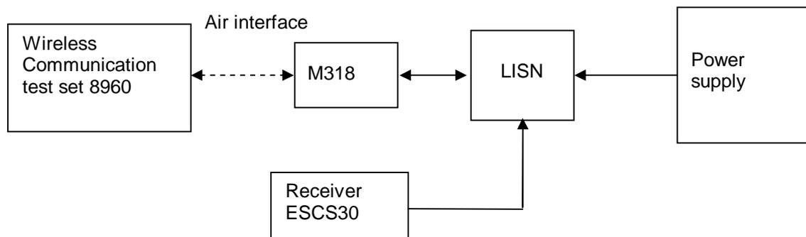
Figure 11. Test Set-up
