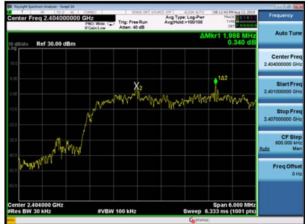
BT UHD 2M 8DPSK, Carrier frequency (MHz): 2440
