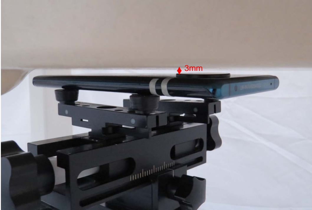
Picture 23: Back Side, the distance from handset to the bottom of the Phantom is 3mm
