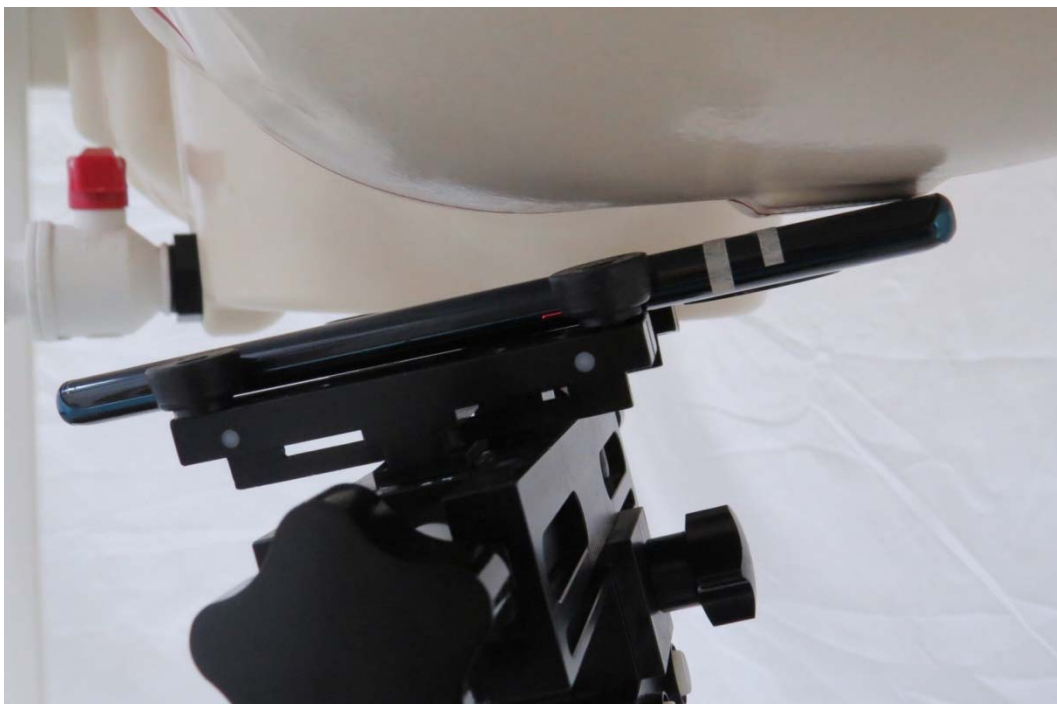
Picture 2: Left Hand Tilt 15 Degree Position
