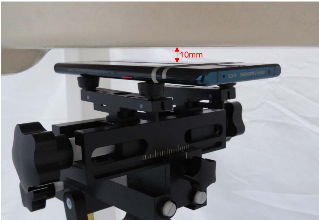
Picture 16: Front Side, the distance from handset to the bottom of the Phantom is 10mm
