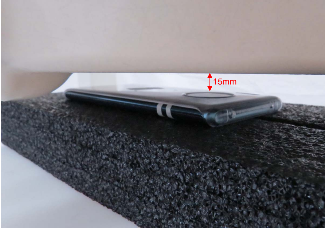
Picture 13: Back Side, the distance from handset to the bottom of the Phantom is 15mm (Mobile phone case (transparent))
