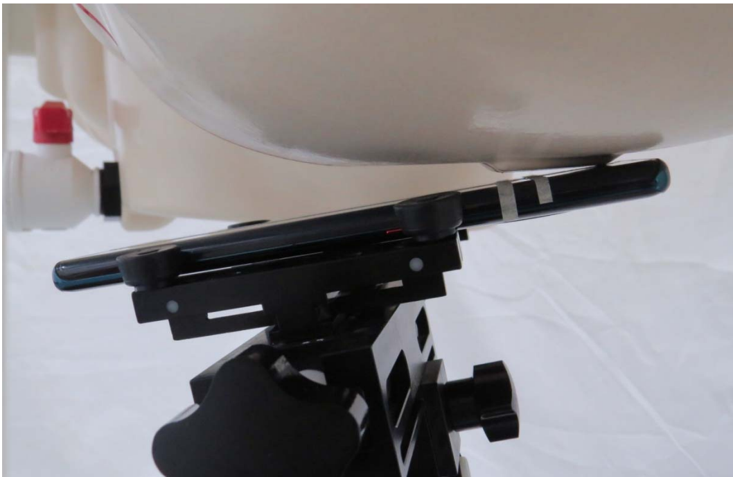
Picture 6: Left Hand Tilt 15 Degree Position (the best acoustic position)
