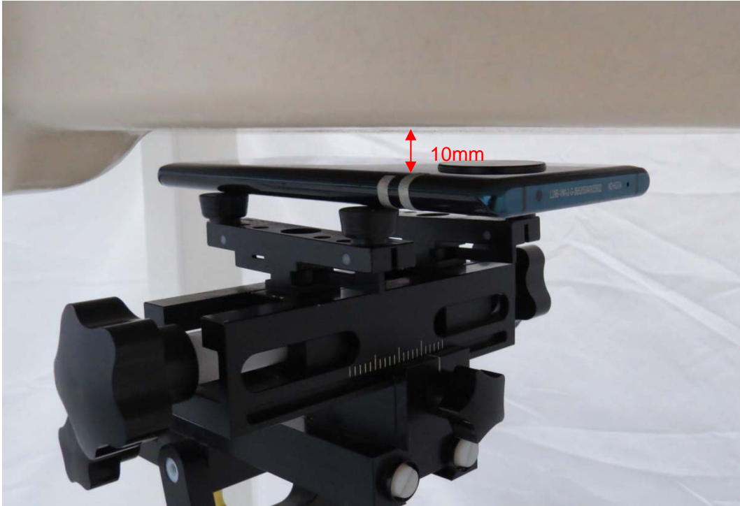
Picture 15: Back Side, the distance from handset to the bottom of the Phantom is 10mm
