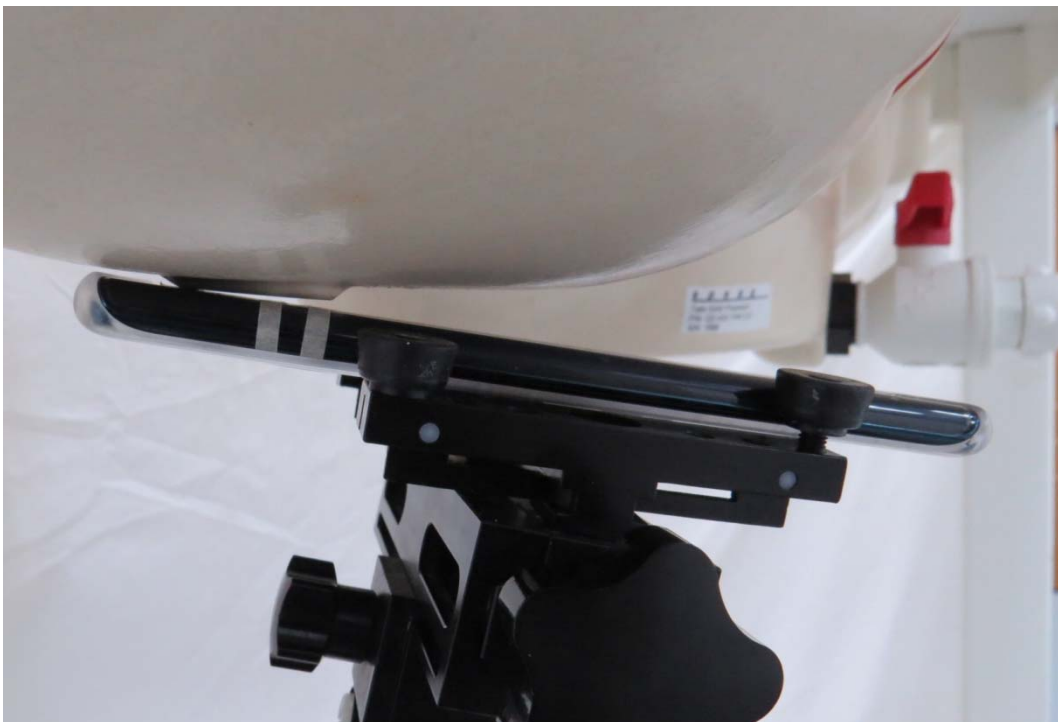
Picture 10: Right Hand Tilt 15 Degree Position (the best acoustic position) (Mobile phone case (transparent))
