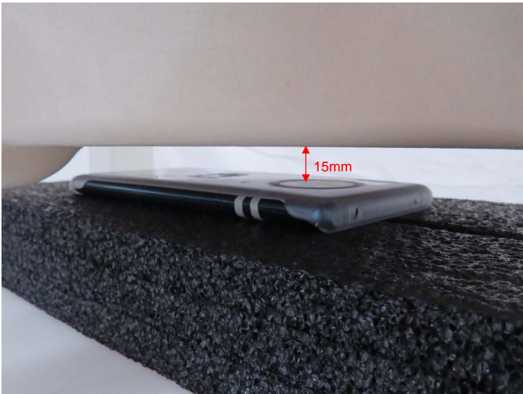
Picture 12: Back Side, the distance from handset to the bottom of the Phantom is 15mm (Mobile phone case (matte))
