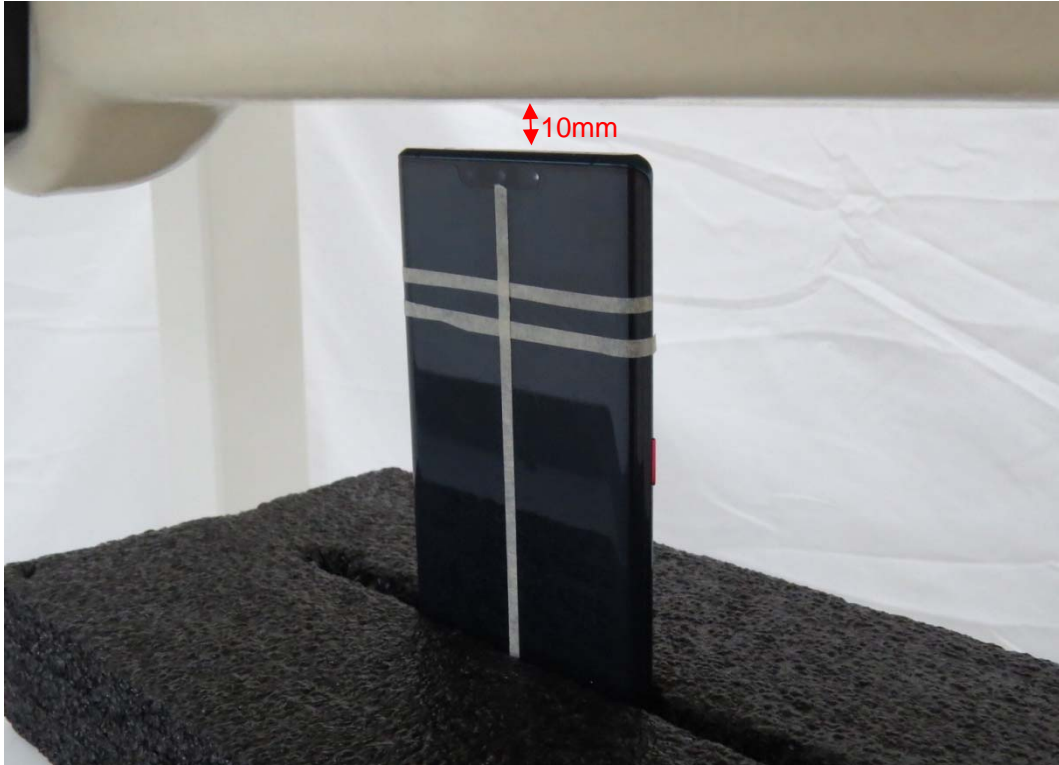
Picture 19: Top Side, the distance from handset to the bottom of the Phantom is 10mm
