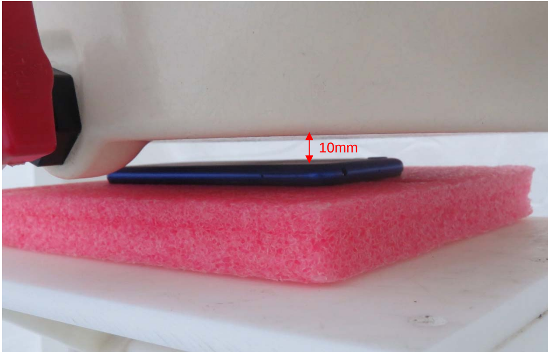
Picture 7: Back Side, the distance from handset to the bottom of the Phantom is 10mm
