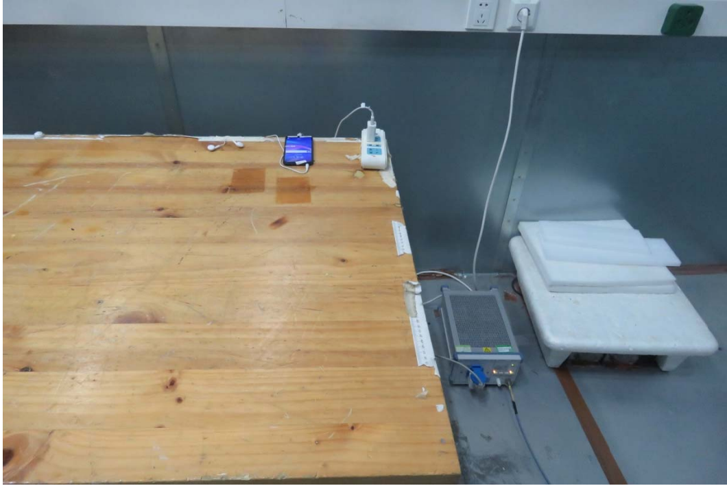
Picture 2 Conducted Emission Test Setup
