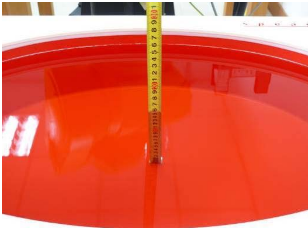
Picture 5: Liquid depth in the flat Phantom (2450 MHz, 15.3cm depth)
