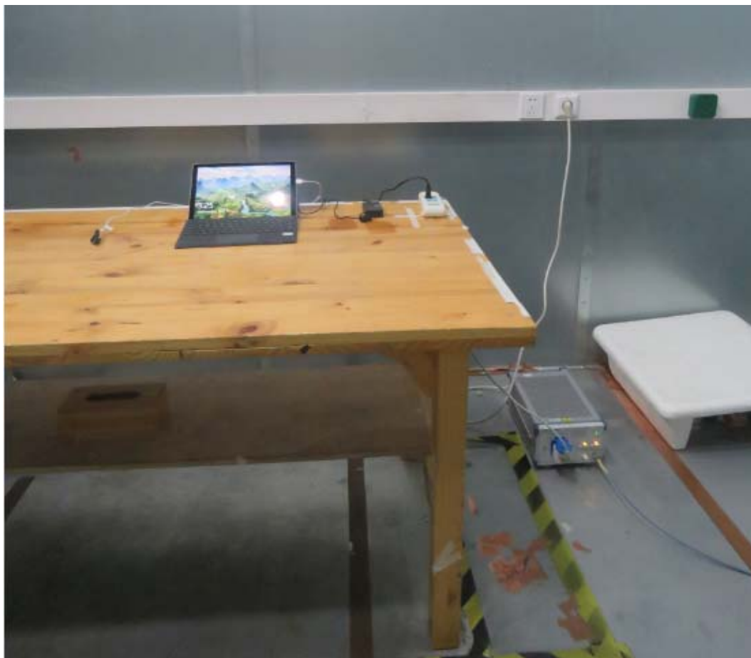
Picture 2 Conducted Emission Test Setup
