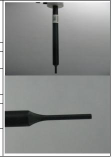
Isotropic E-Field Probe EX3DV4 for Dosimetric Measurements
