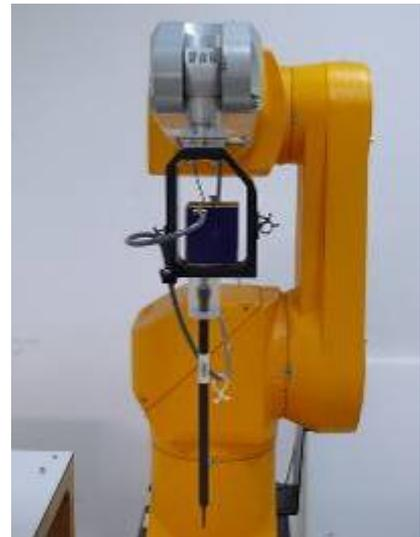
Figure 3. EX3DV4 E-field probe
