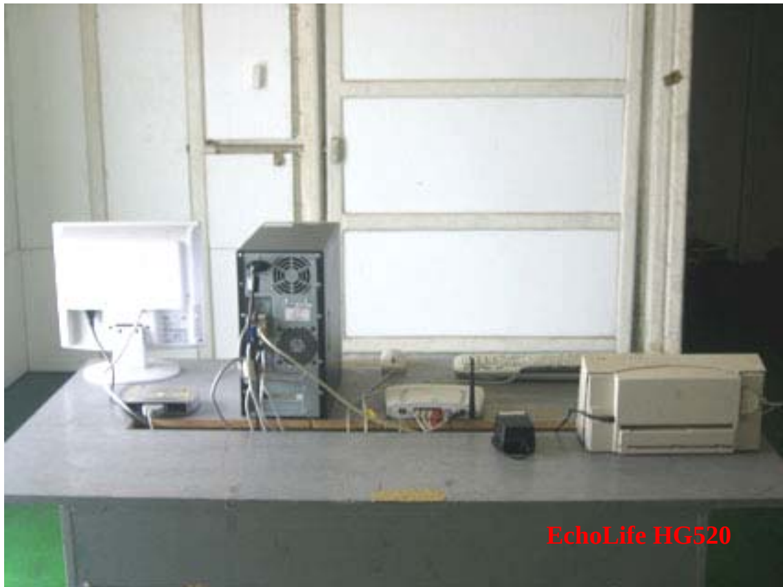
Photo 2: Radiated Emission Test set-up photo
