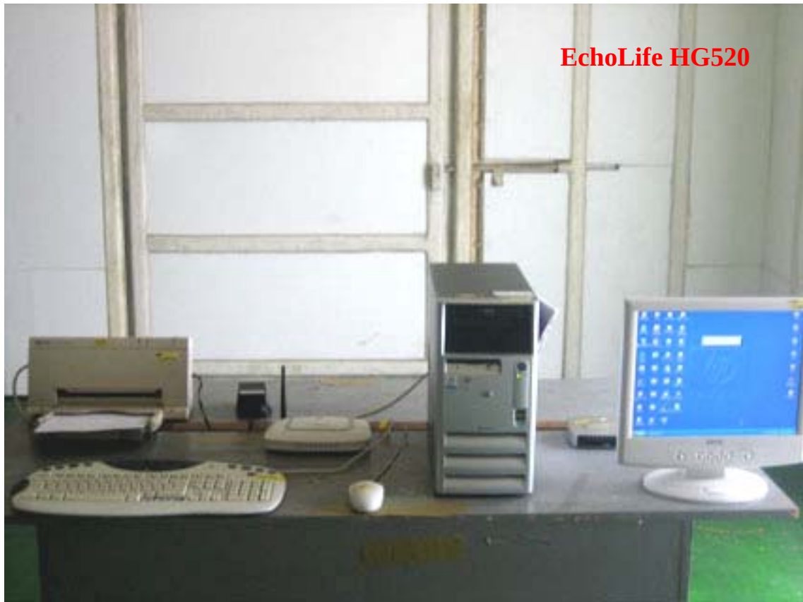
Photo 1: Radiated Emission Test set-up photo
