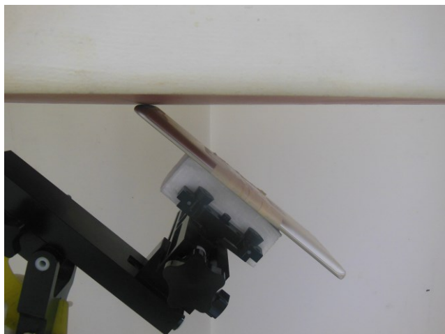
Curved Surface of Bottom Edge Test Separation 0 mm
