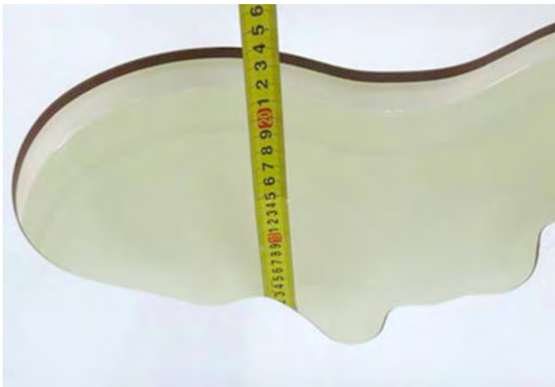
Picture 7: liquid depth in the head Phantom (1900 MHz, 15.3cm depth)
