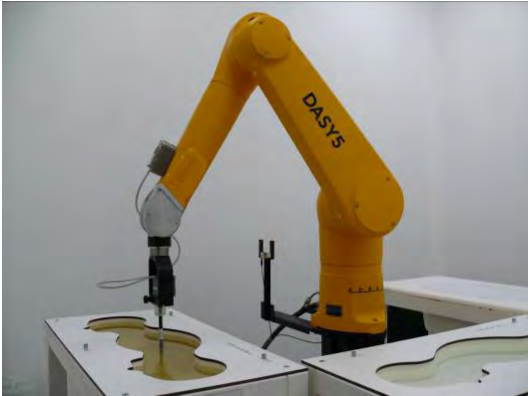
Picture 1: Specific Absorption Rate Test Layout
