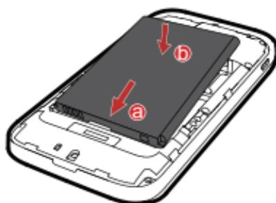
1. Angle the edge labeled **a** (with the contacts) into the bottom end of the battery compartment.
