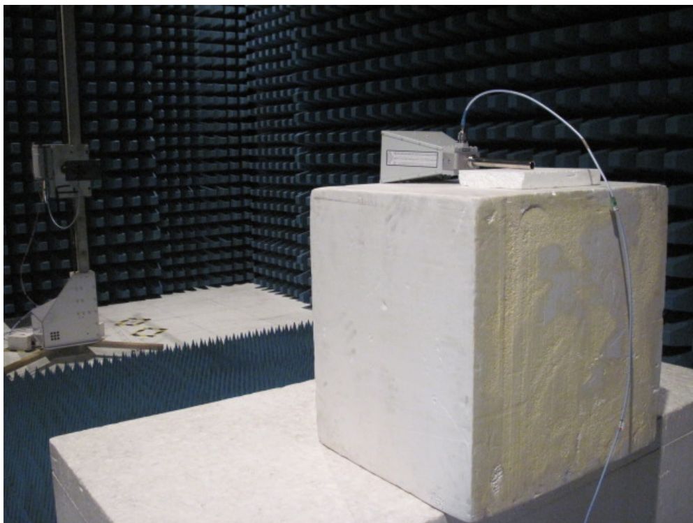
Description: Substitution Antenna for EIRP Test
