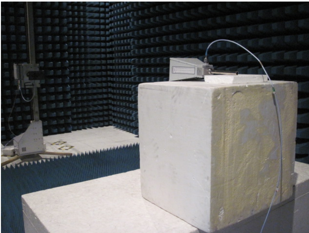
Description: Substitution Antenna for EIRP Test
