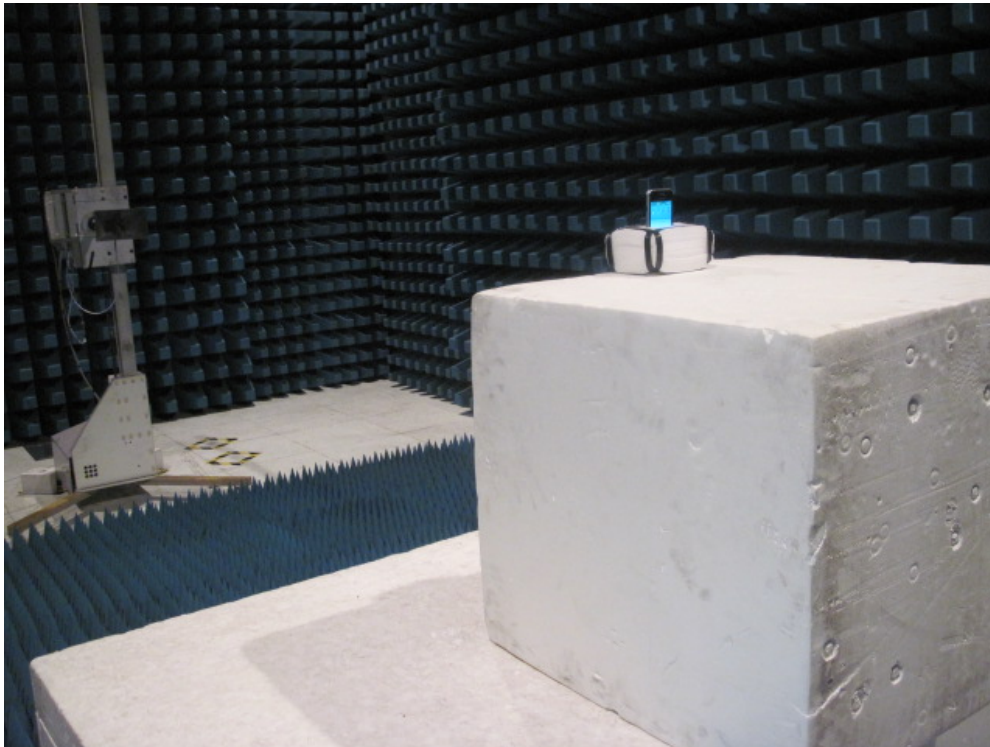
Description: EIRP Test Setup
