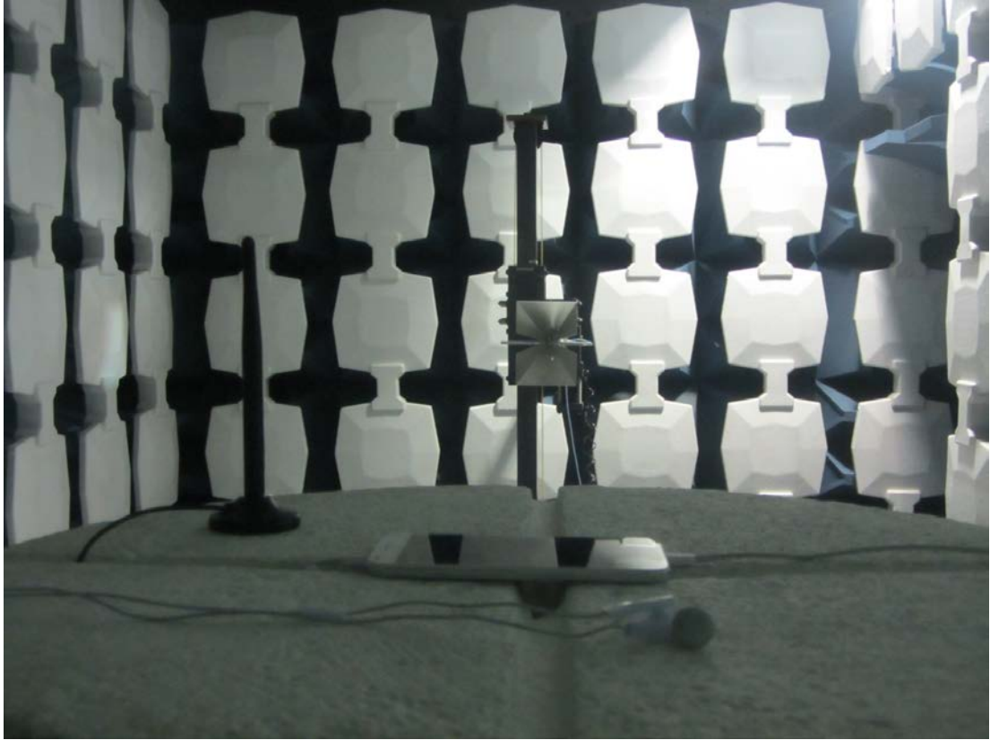
Radiated Spurious Emission (3GHz to18GHz)
