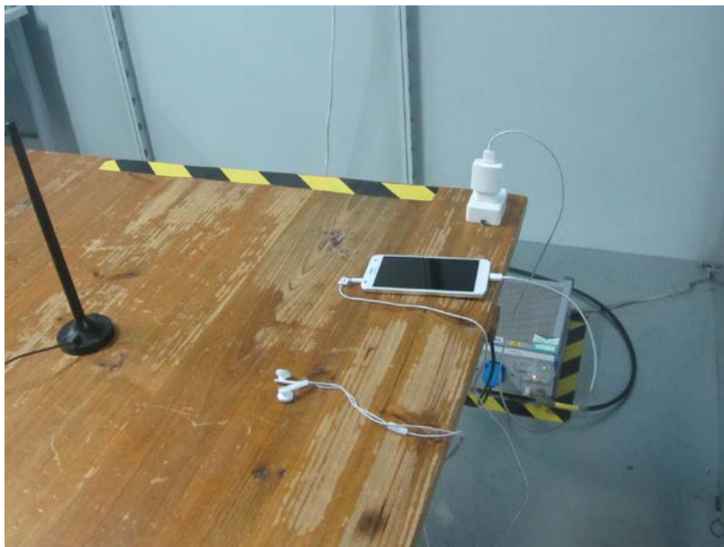
Conducted Emissions for AC Ports
