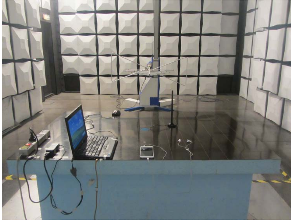
Radiated Spurious Emission (below 1GHz)
