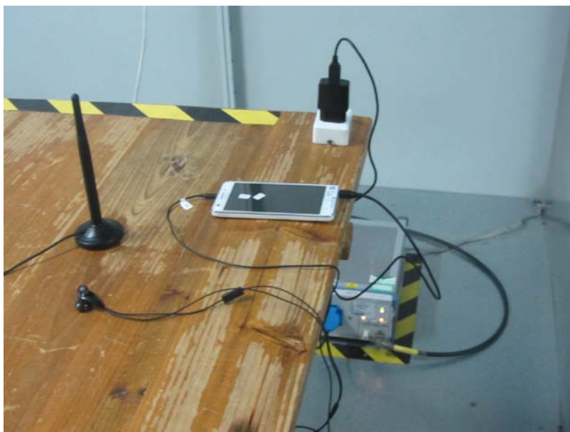
Conducted Emissions with AC Ports
