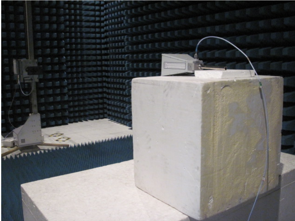
Description: Substitution Antenna for EIRP Test
