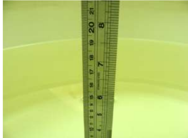
Fig 6.2 Photo of Liquid Height for Body SAR
