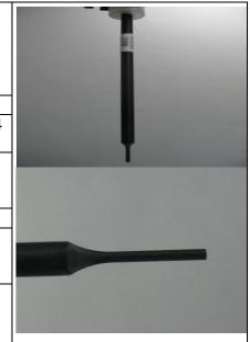
Isotropic E-Field Probe EX3DV4 for Dosimetric Measurements
