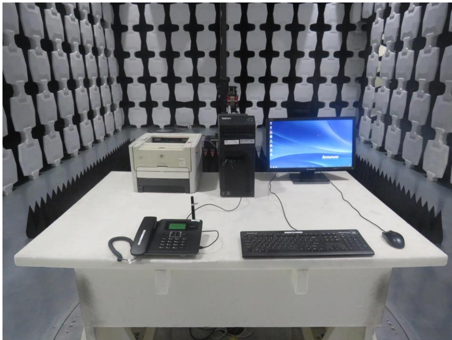
2. Radiated Emissions (Part 15B PC mode)(Above 1GHz)
