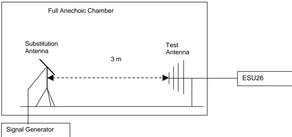
Figure 1. Test Set-up
