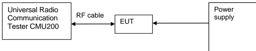
Figure 2. Test Set-up
