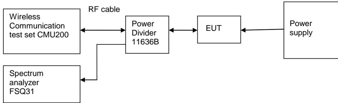
Figure 5. Test Set-up
