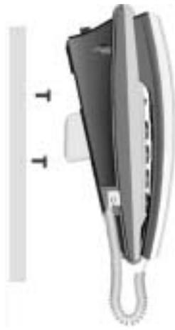
Figure 4-9 FWT vertical placement
