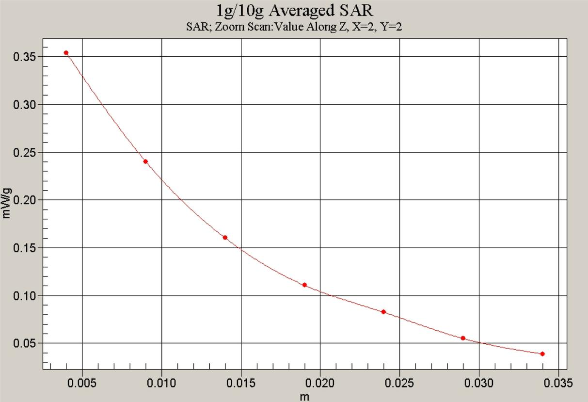
Fig.14 Z-Scan at power reference point
