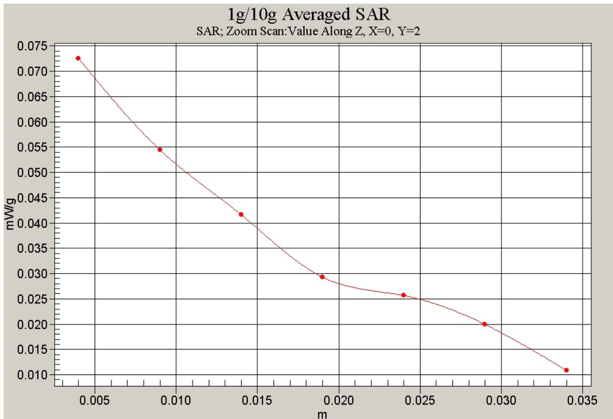
Fig.36 Z-Scan at power reference point
