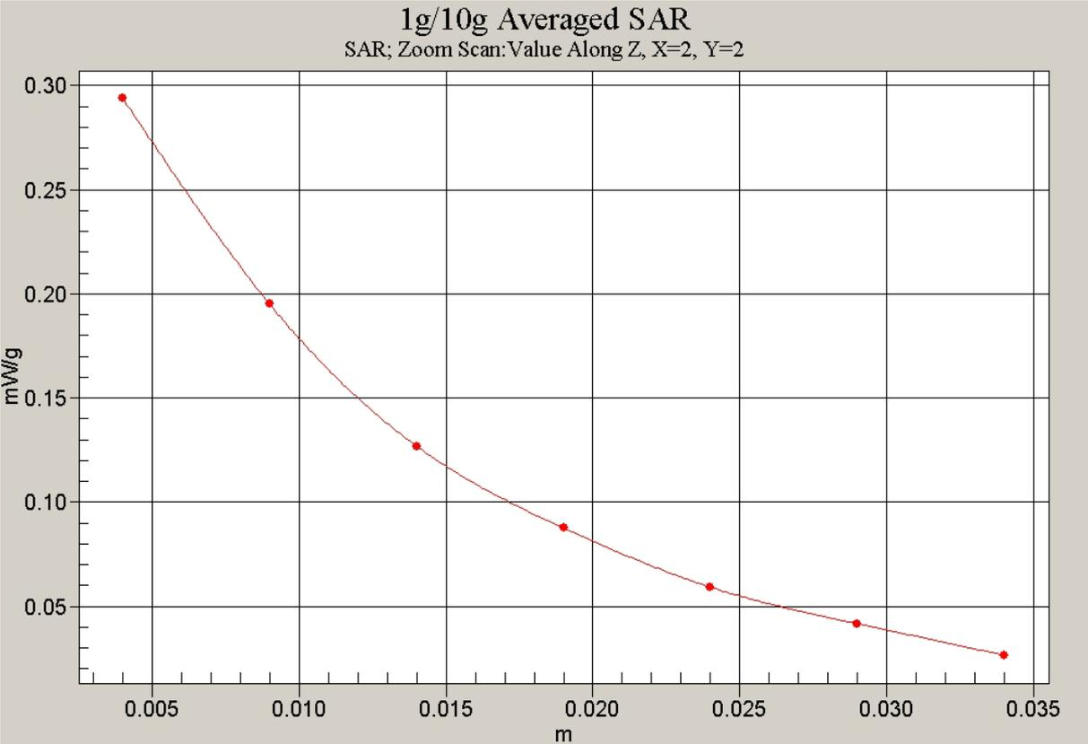
Fig.34 Z-Scan at power reference point
