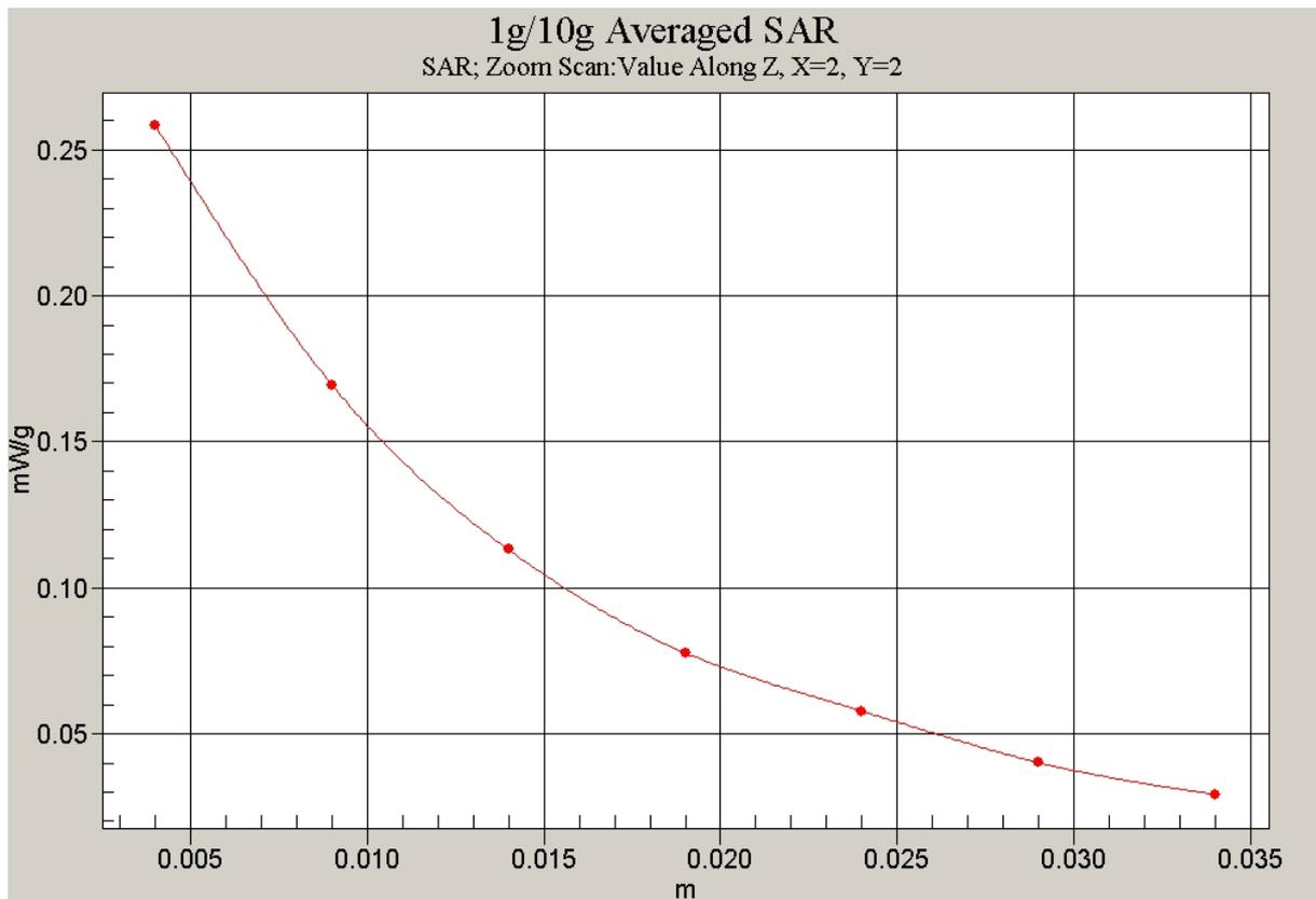
Fig.54 Z-Scan at power reference point
