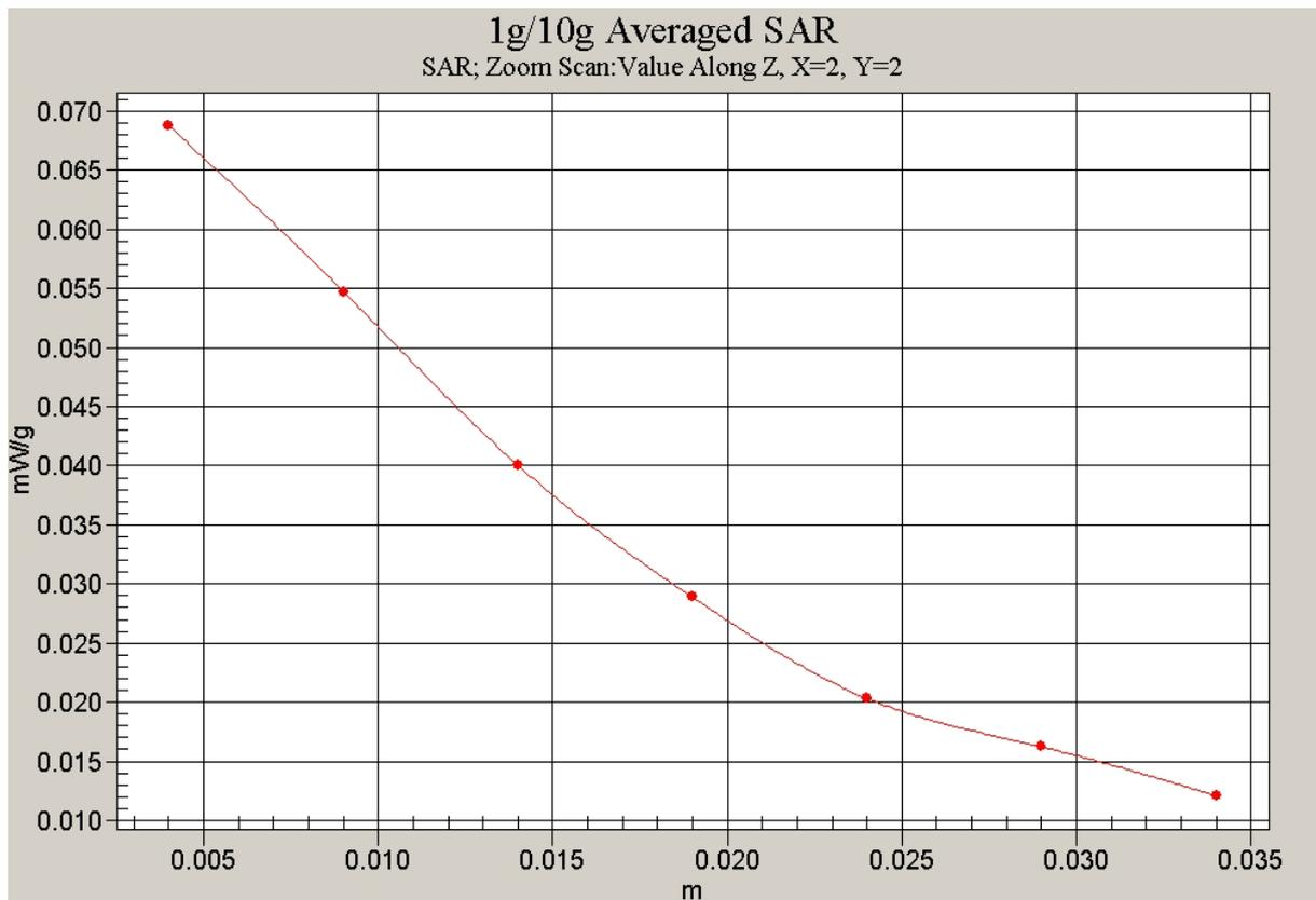
Fig.42 Z-Scan at power reference point
