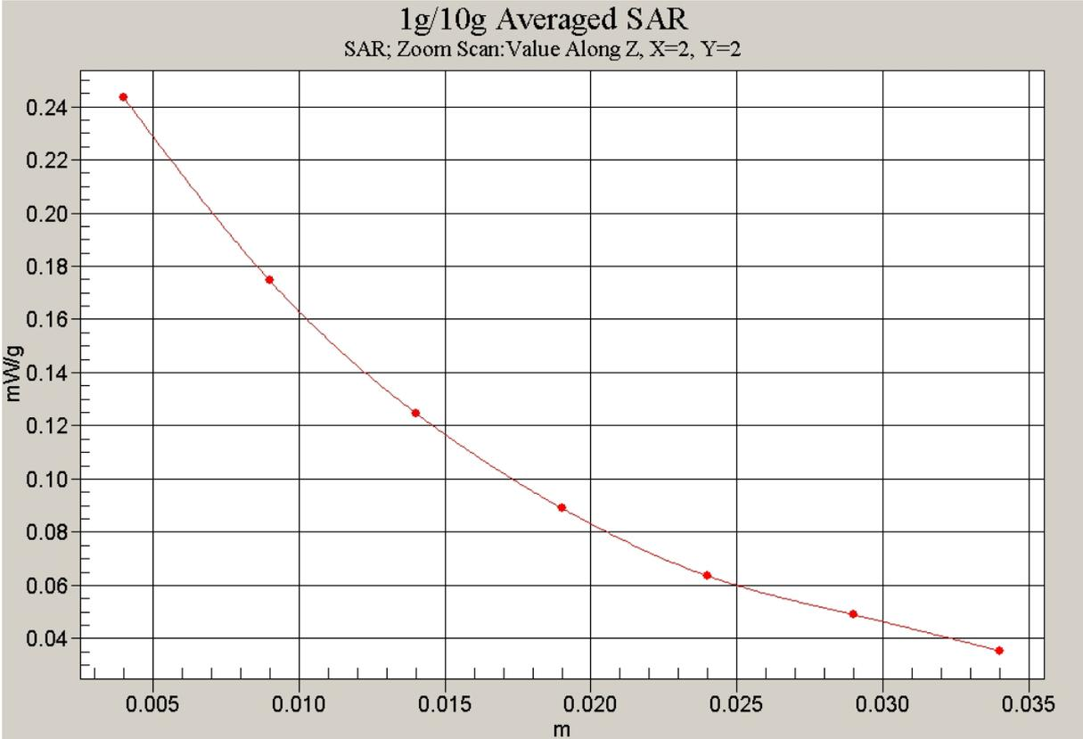
Fig.38 Z-Scan at power reference point
