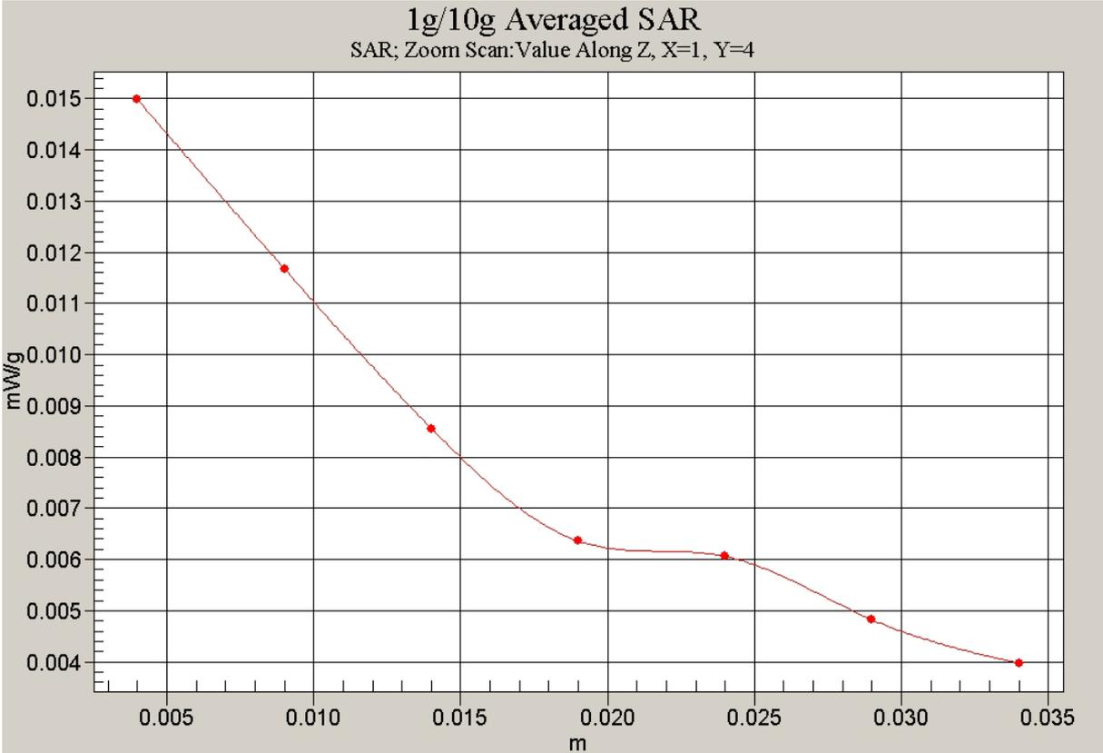
Fig.20 Z-Scan at power reference point
