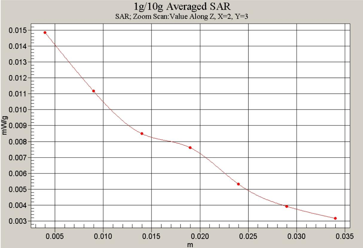
Fig.30 Z-Scan at power reference point
