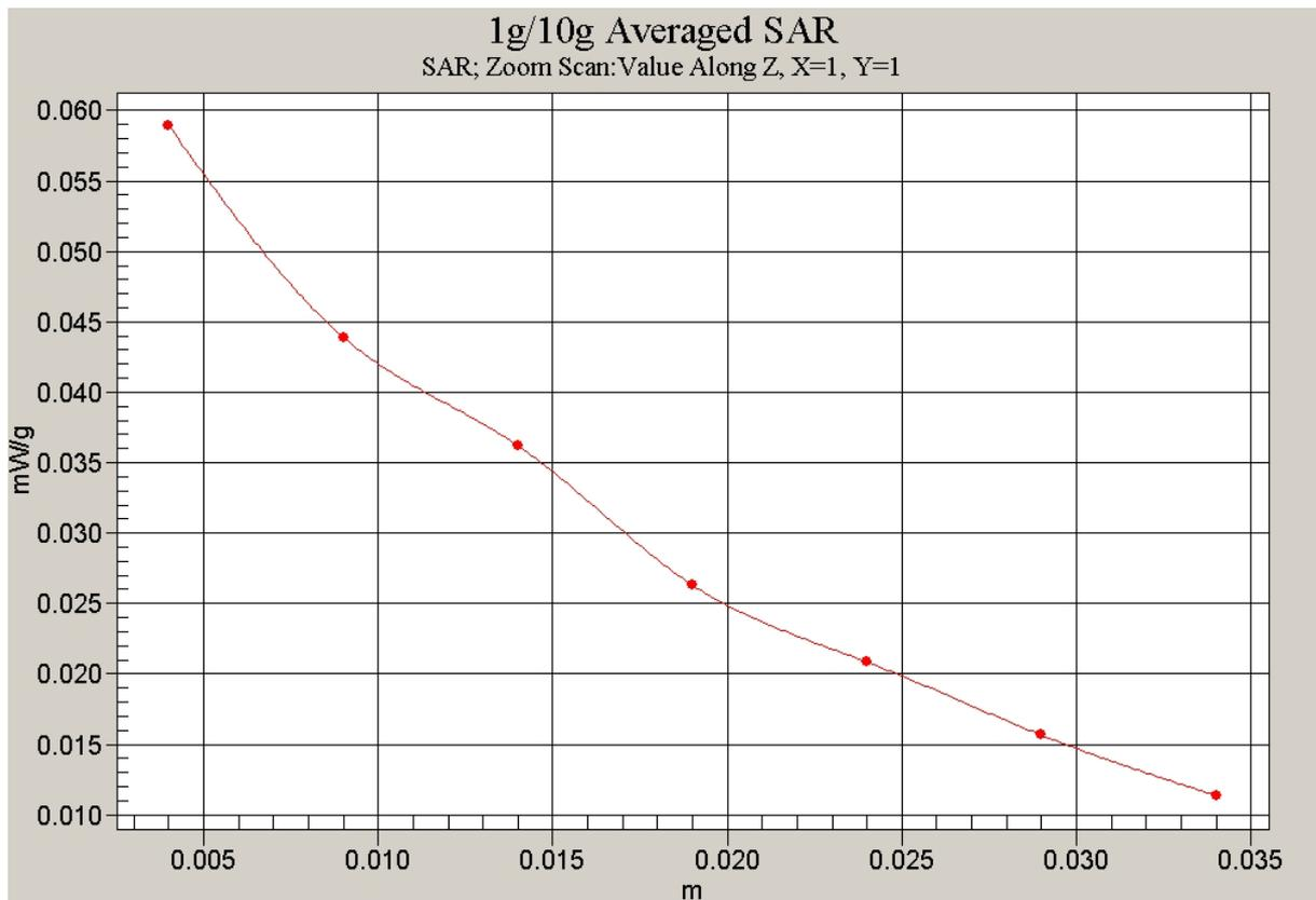
Fig.56 Z-Scan at power reference point
