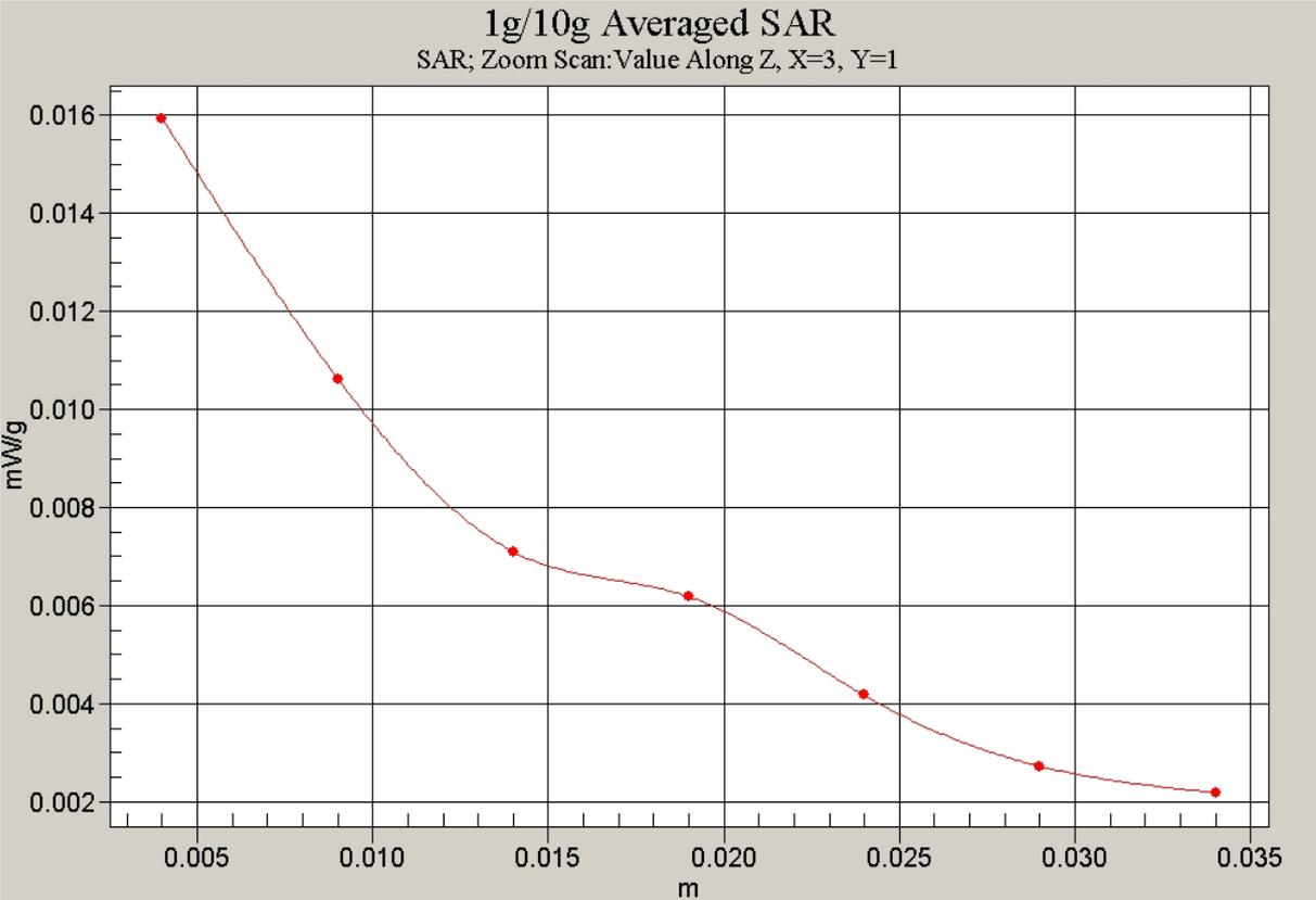
Fig.48 Z-Scan at power reference point
