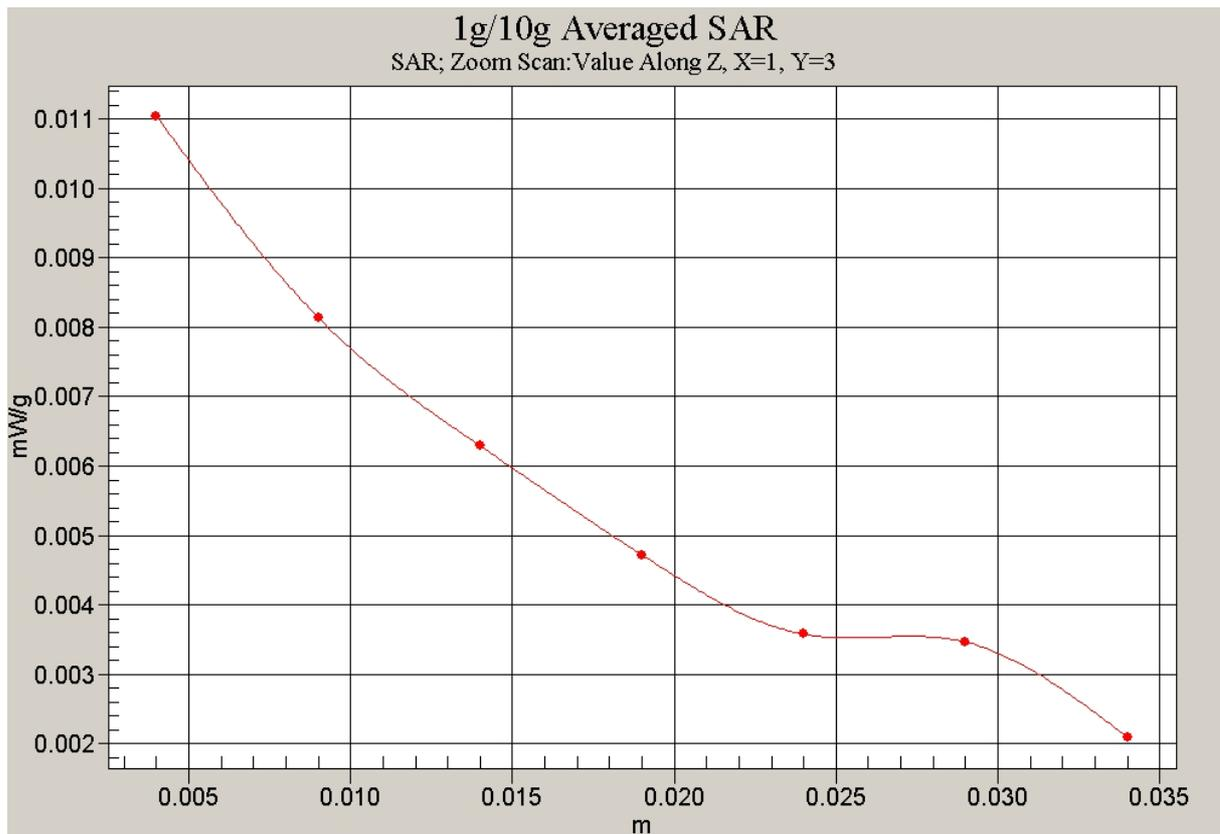
Fig.6 Z-Scan at power reference point
