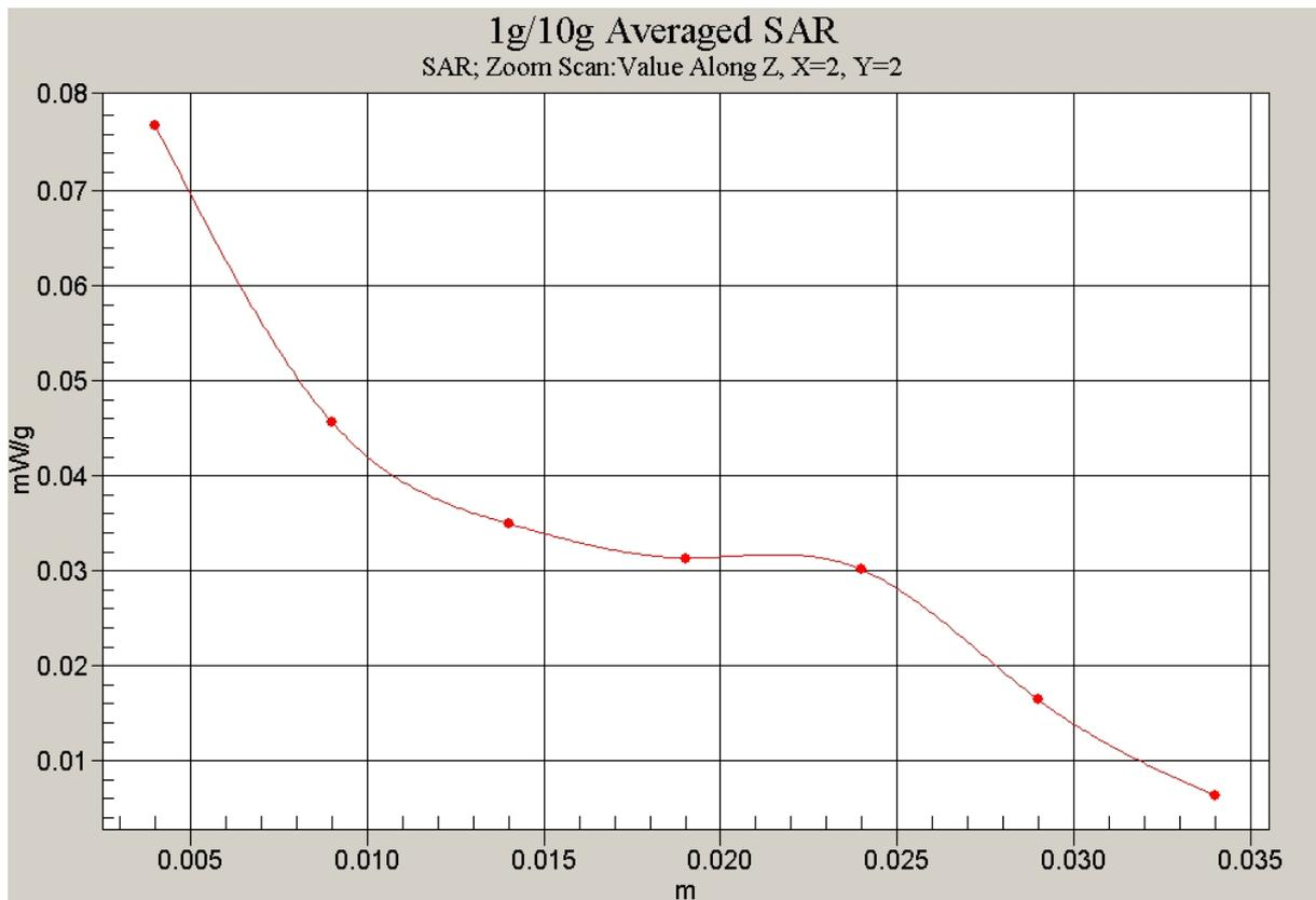
Fig.66 Z-Scan at power reference point
