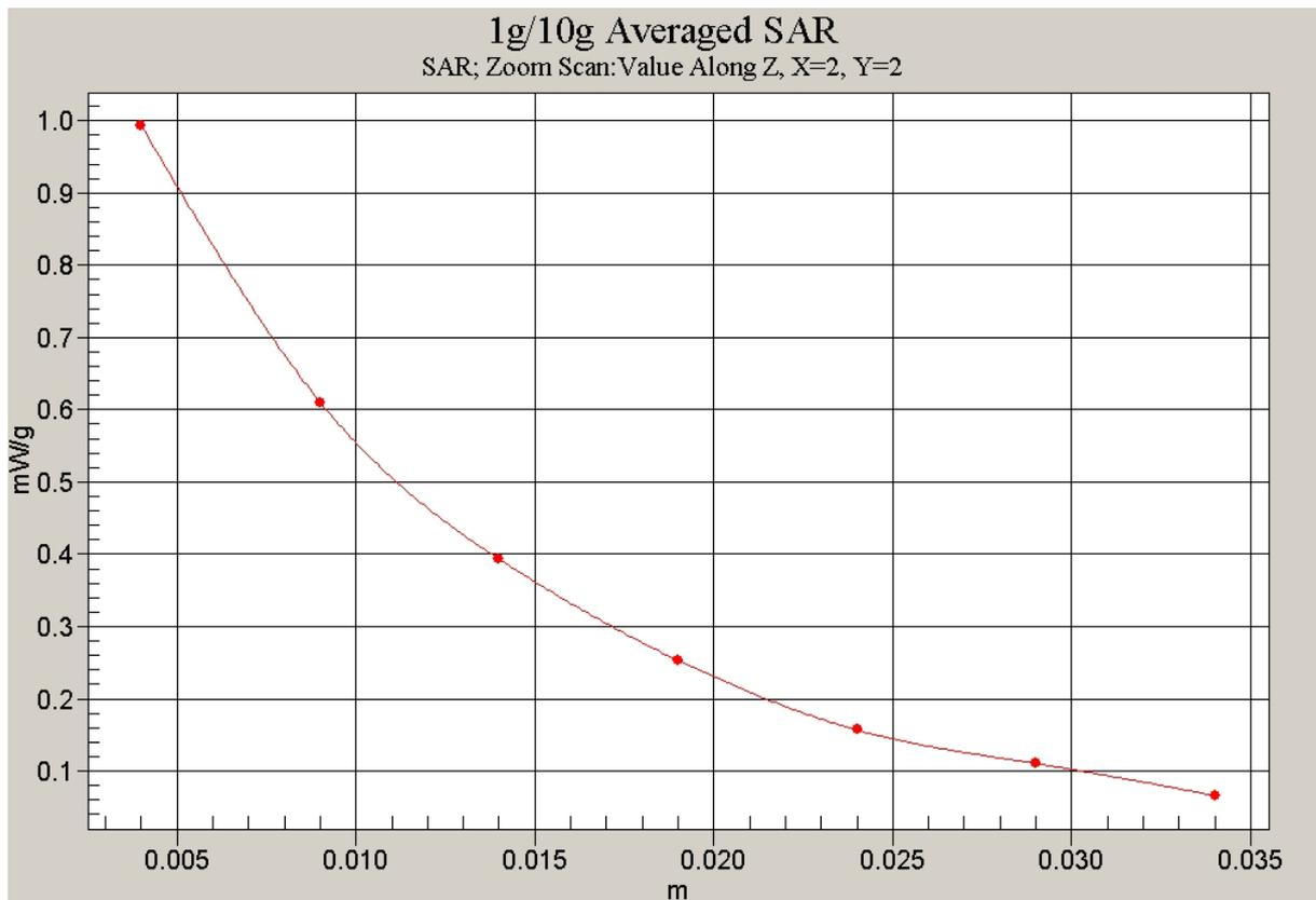
Fig.70 Z-Scan at power reference point
