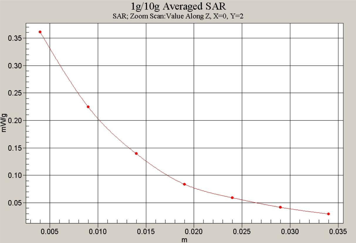
Fig.68 Z-Scan at power reference point
