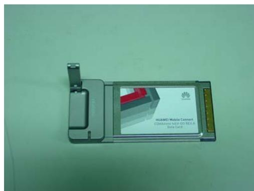
Picture 1-a: Front side of the EUT (antenna folded)    Picture 1-b: Back Side of the EUT (antenna unfolded)
