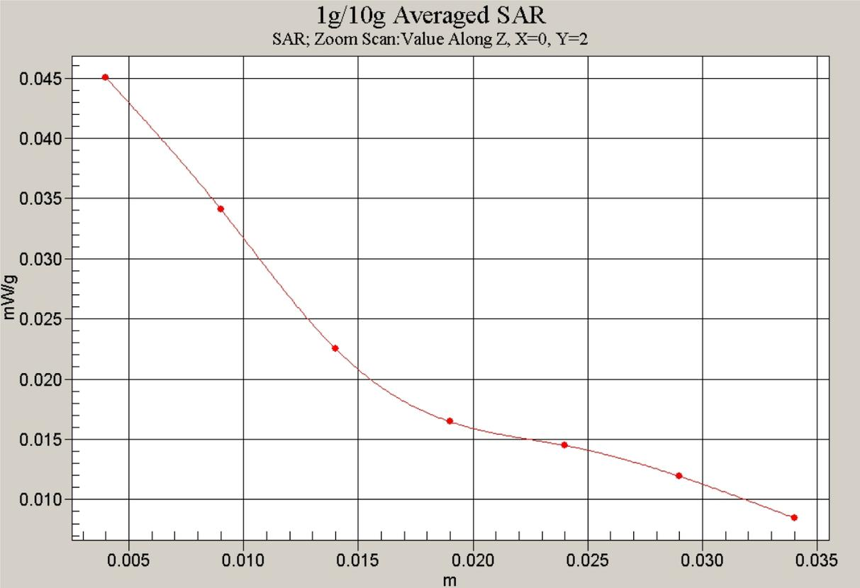
Fig.8 Z-Scan at power reference point
