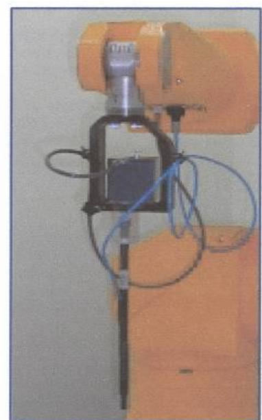
Figure 3 ET3DV6 E-field probe
