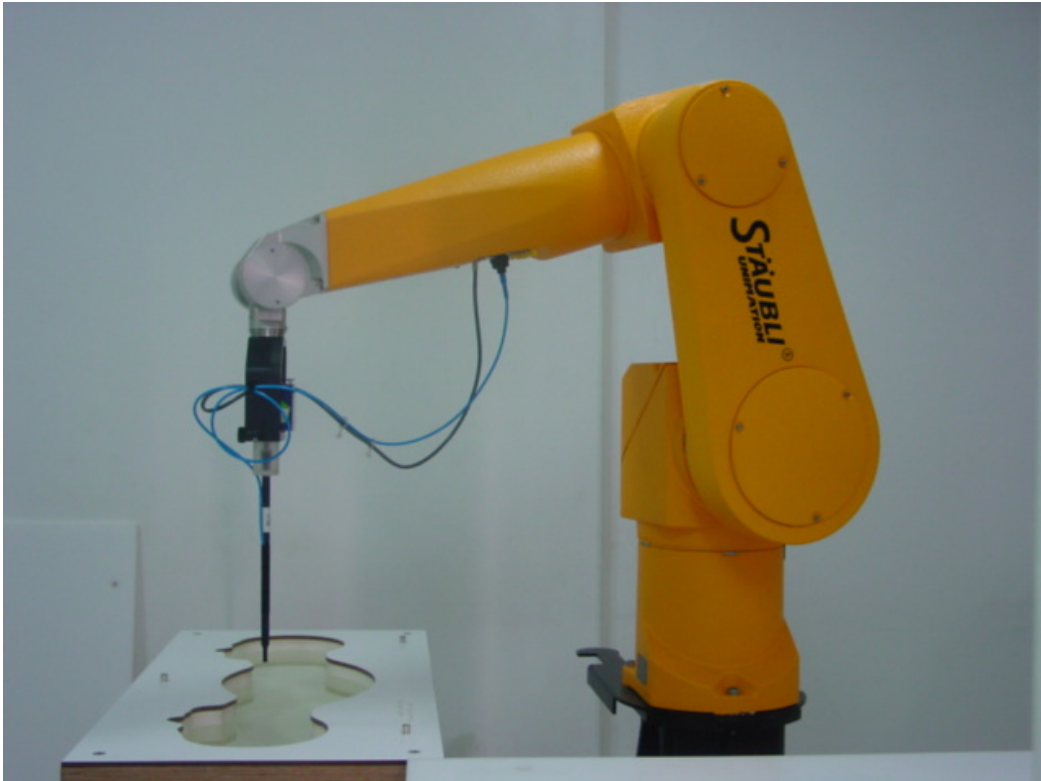
Picture 2 Specific Absorption Rate Test Layout
